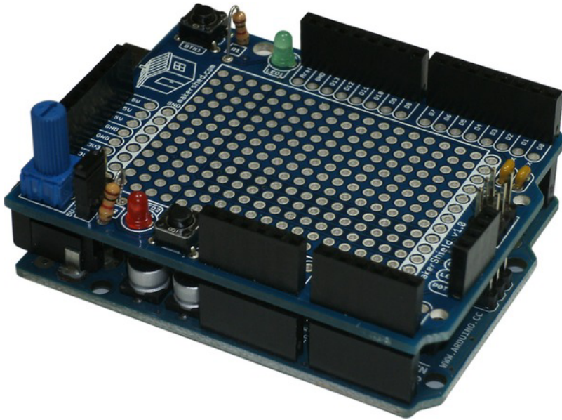
Figure 1-6. The Maker Shield is a full-size Arduino shield that completely covers the Arduino underneath. Stacking connectors allow all the signals from the expansion connector to be replicated above, allowing another shield to be installed on top. The “sea of holes” in the middle is for mounting additional components, extending the functionality of your Arduino.
