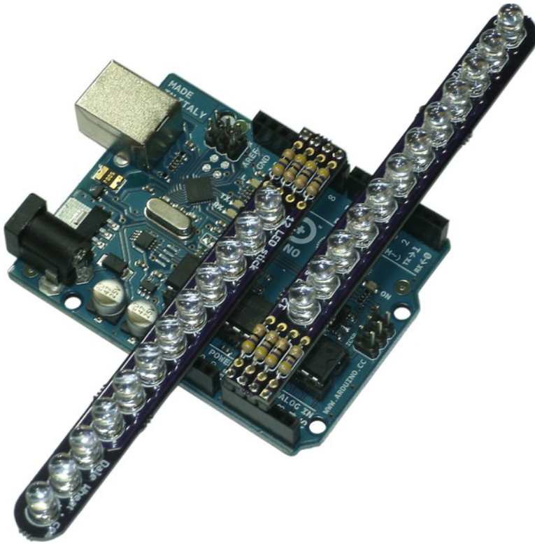
Figure 1-7. Smaller shields that use only a few I/O lines can be installed in the expansion connectors. The use of multiplexed connections allows up to a dozen LEDs to be individually addressed while only requiring four dedicated control lines from the Arduino.
