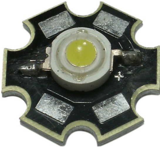
Figure 8-5. A 1W white LED, attached to an aluminum-core PCB as a heatsink
