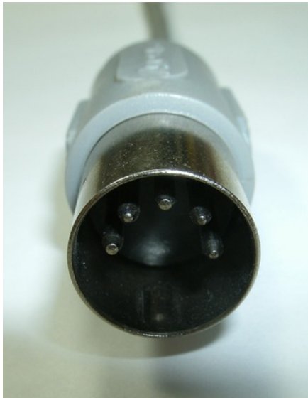
Figure 12-9. The business end of a MIDI cable. The pins are numbered, left to right: 1, 4, 2, 5, 3. There is an alignment notch in the bottom half of the shield.
