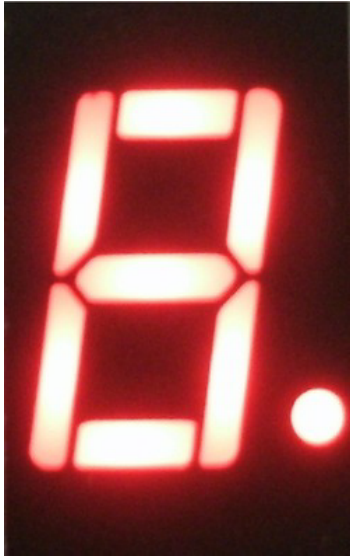
Figure 8-17. A seven-segment LED array can represent the numerals from 0–9, and a few letters, too. An eighth LED forms a right-hand decimal point.
