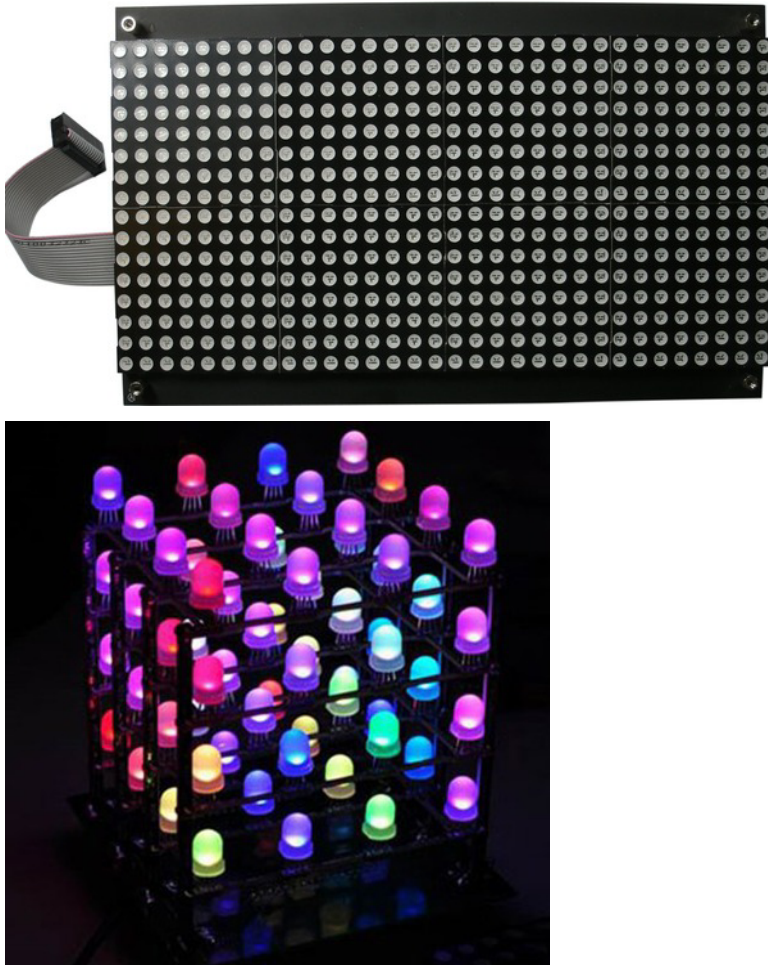
Figure 8-16. A 32 \times 16 bicolor (red + green) LED array with embedded drivers from Sure Electronics (top) and the 3D 4 \times 4 \times 4 RGB LED Cube kit from Seeed Studio (bottom).
