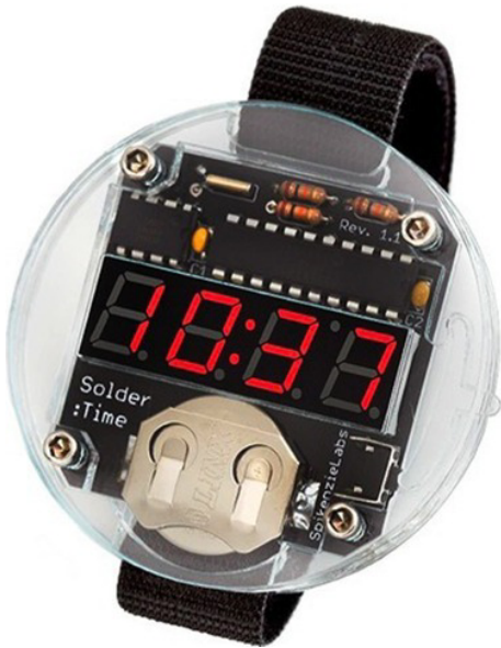
Figure 8-20. The Solder : Time watch kit from SpikenzieLabs turns on only one segment at a time to conserve battery power, while still presenting a very readable LED display.
