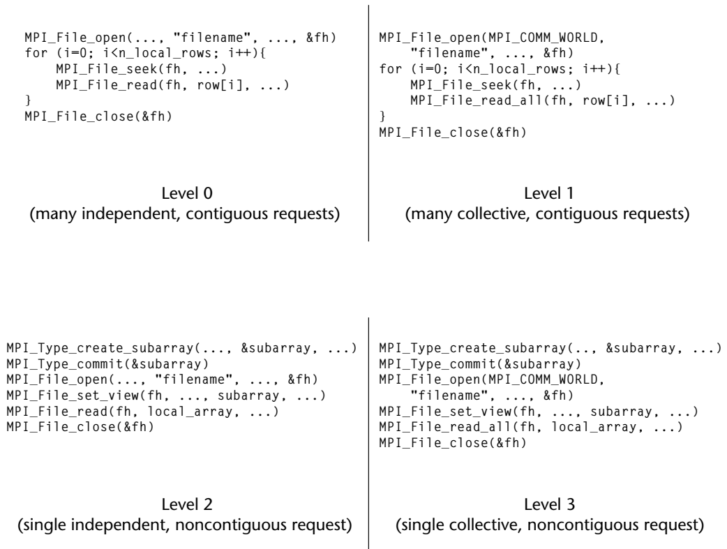
Figure 11.8 Pseudocode that shows four ways of accessing the data in Figure 11.3 with MPI-IO.
