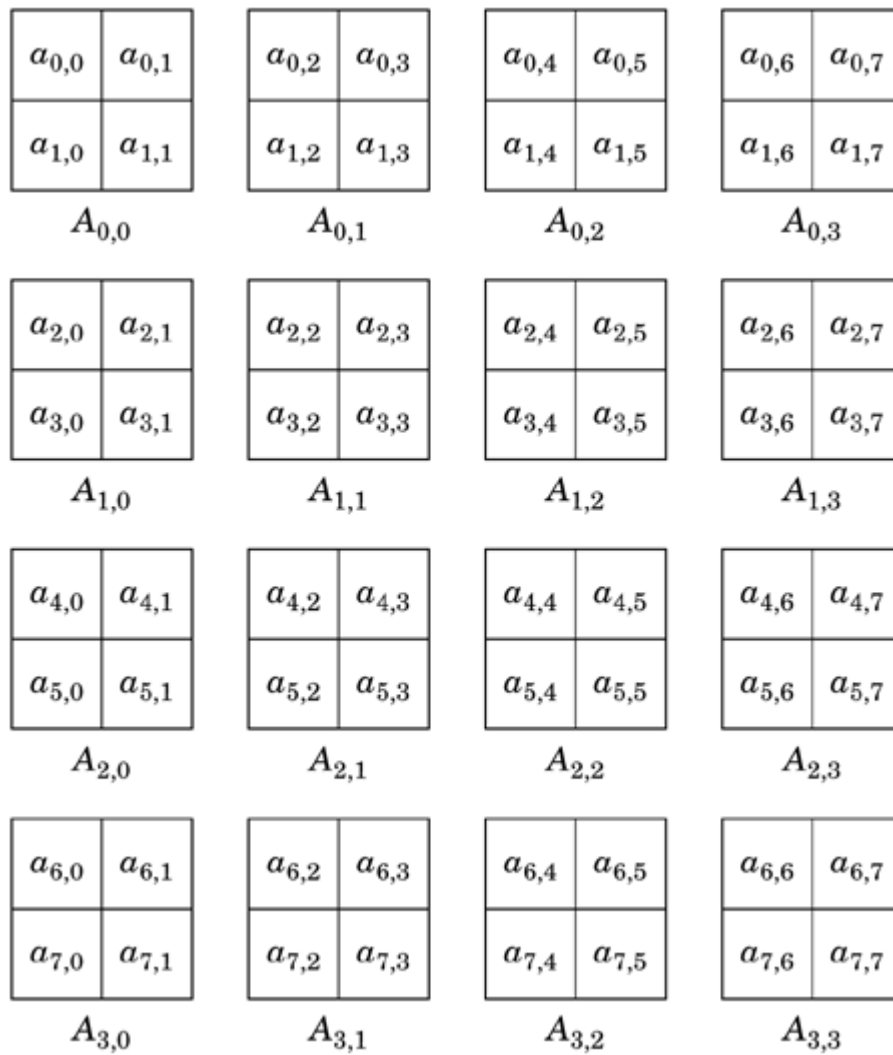
Figure 5.53. 2D block-cyclic distribution of A onto four UEs, part 1: Decomposing A
