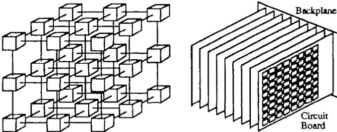
Figure 12.1. 3D and 2.5D physical realizations of a 3D mesh.
