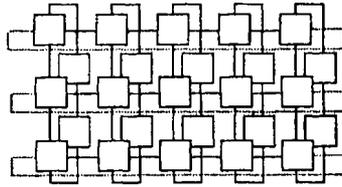
Figure 9.2. A  $5 \times 5$  torus folded along its columns. Folding this diagram along the rows will produce a layout with only short links.
