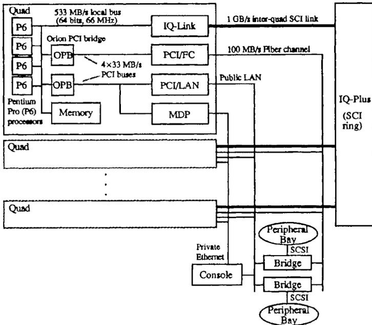
Figure 21.10. The architecture of Sequent NUMA-Q 2000.
