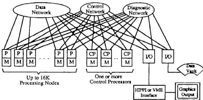
Figure 22.7. The overall structure of CM-5.
