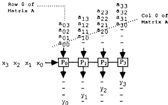
Figure 11 .1. Matrix–vector multiplication on a linear array.
