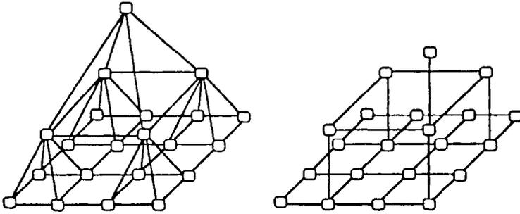
Figure 12.12. The relationship between pyramid and 2D multigrid architectures.
