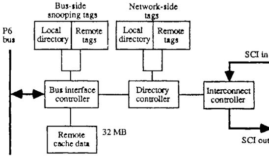
Figure 21.11. Block diagram of the IQ-Link board.
