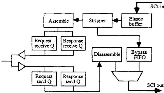
Figure 21.12. Block diagram of IQ-Link's interconnect controller.
