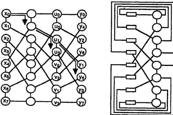
Figure 8.12. FFT network variant and its shared-hardware realization.
