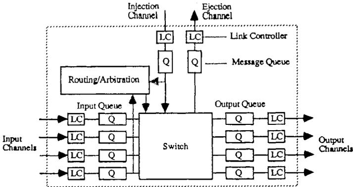
Figure 22.1. The structure of a generic router.
