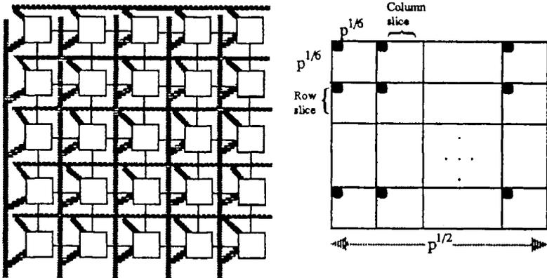
Figure 12.8. Mesh with row/column buses and semigroup computation on it.
