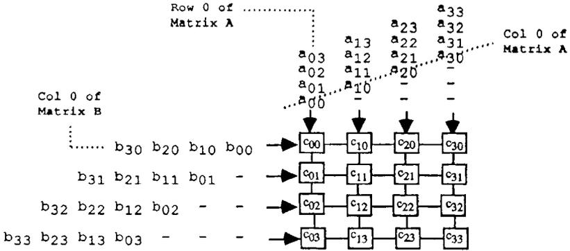
Figure 11.2. Matrix–matrix multiplication on a 2D mesh.
