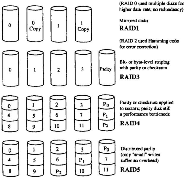
Figure 18.8. Alternative data organizations on redundant disk arrays.
