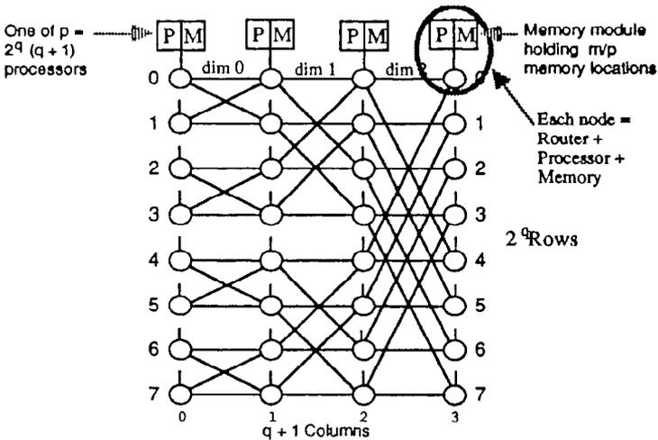
Figure 17.2. Butterfly distributed-memory machine emulating the PRAM.
