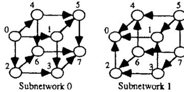
Figure 14.11. Partitioning a 3-cube into subnetworks for deadlock-free routing.
