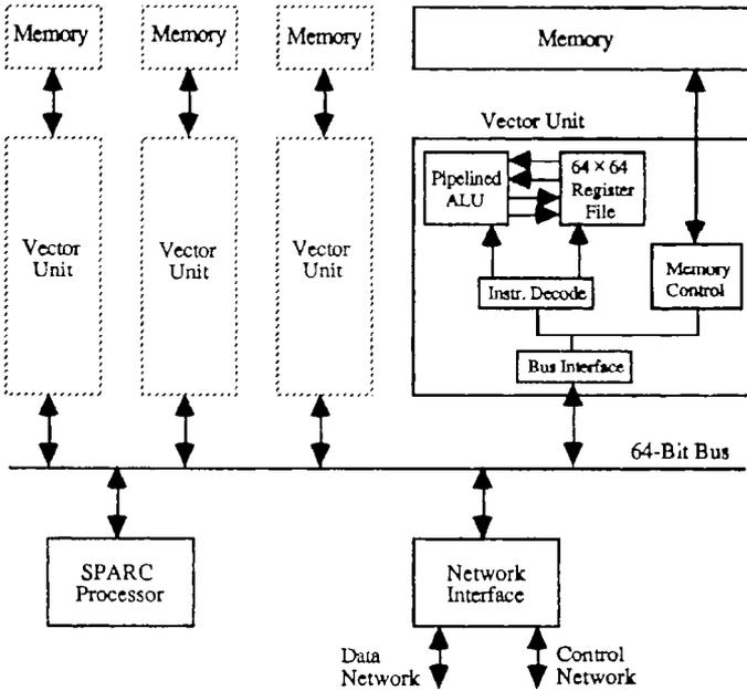
Figure 22.8. The components of a processing node in CM-5.
