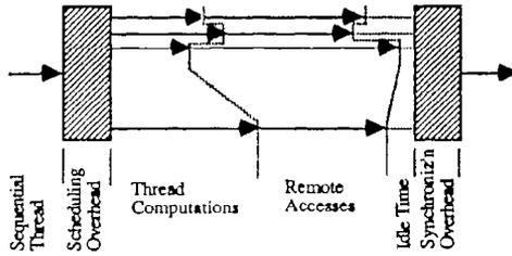
Figure 18.5. The concept of multithreaded parallel computation.
