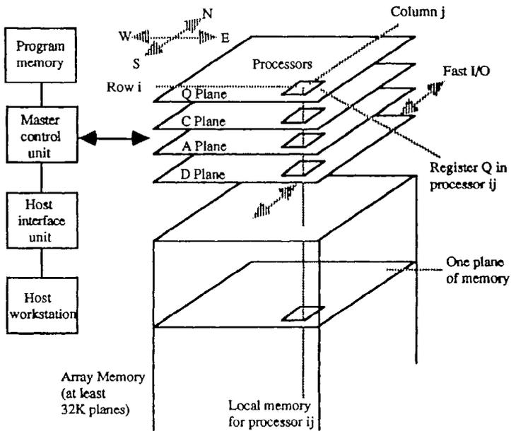
Figure 23.7. The high-level architecture of DAP system.
