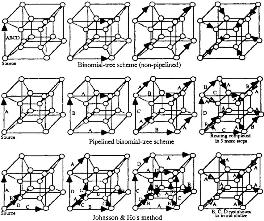
Figure 14.10. Three hypercube broadcasting schemes as performed on a 4-cube.
