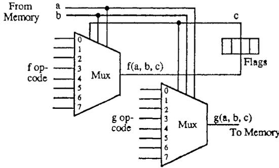
Figure 23.9. The bit-serial ALU of CM-2.
