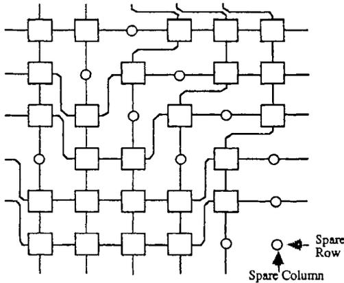
Figure 19.6. A 5 × 5 working array salvaged from a 6 × 6 redundant mesh through reconfiguration switching.
