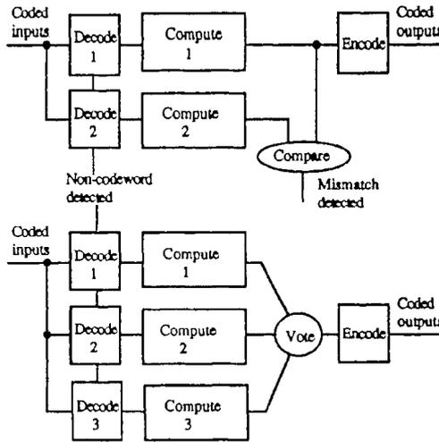
Figure 19.8. Fault detection or tolerance with replication.
