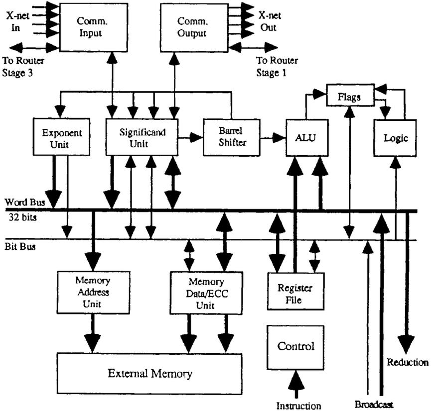
Figure 23.12. Processor architecture in MasPar MP-2.
