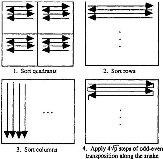
Figure 9.10. Graphical depiction of the first recursive algorithm for sorting on a 2D mesh based on four-way divide and conquer.
