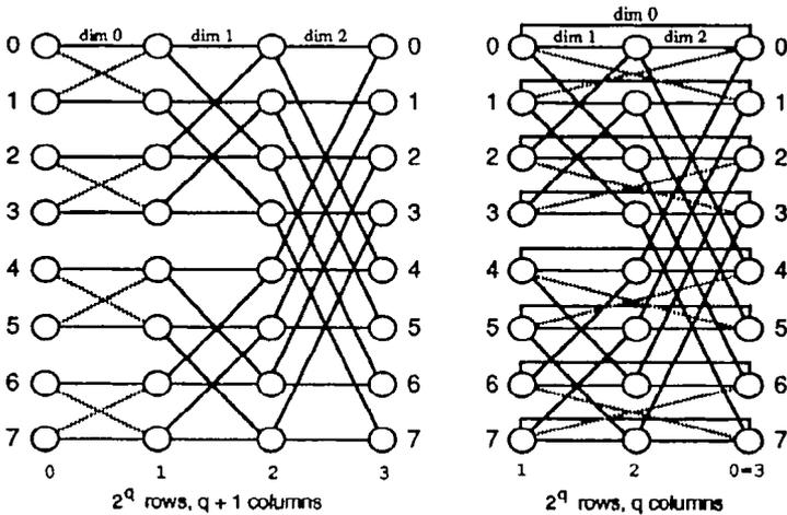
Figure 15.4. Butterfly and wrapped butterfly networks.
