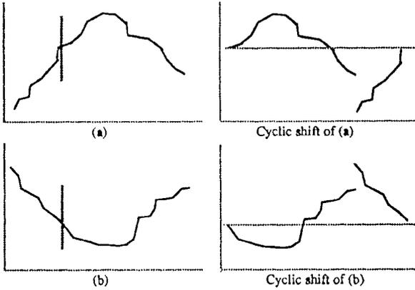
Figure 14.1. Examples of bitonic sequences.
