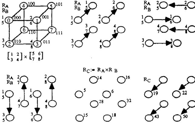
Figure 13.12. Multiplying two  $2 \times 2$  matrices on a 3-cube.
