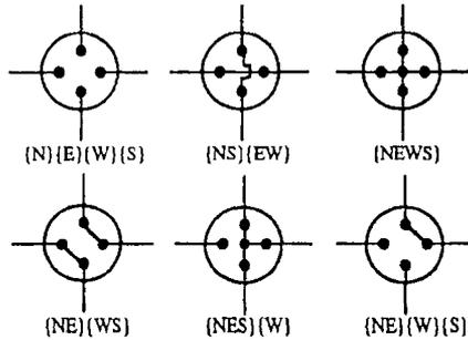
Figure 12.10. Some processor states in a reconfigurable mesh.
