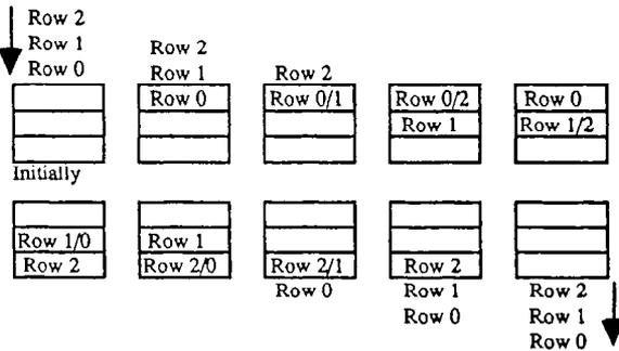
Figure 11.16. Transitive closure algorithm on a 2D mesh.
