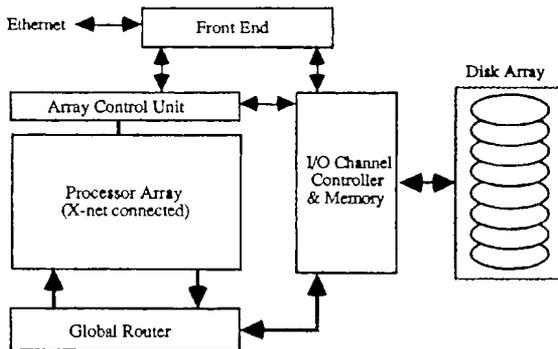
Figure 23.10. The architecture of MasPar MP-2.
