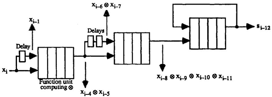
Figure 8.5. High-throughput prefix computation using a pipelined function unit.
