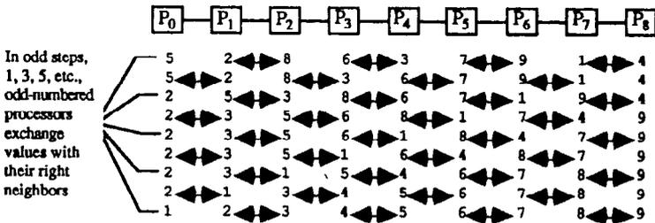
Figure 2.10. Odd-even transposition sort on a linear array.
