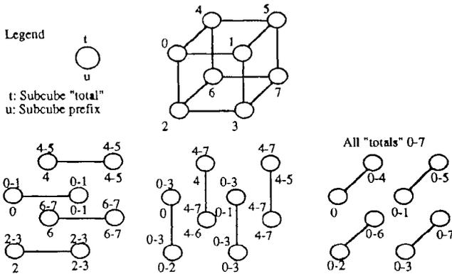
Figure 13.9. Parallel prefix computation on a 3-cube.
