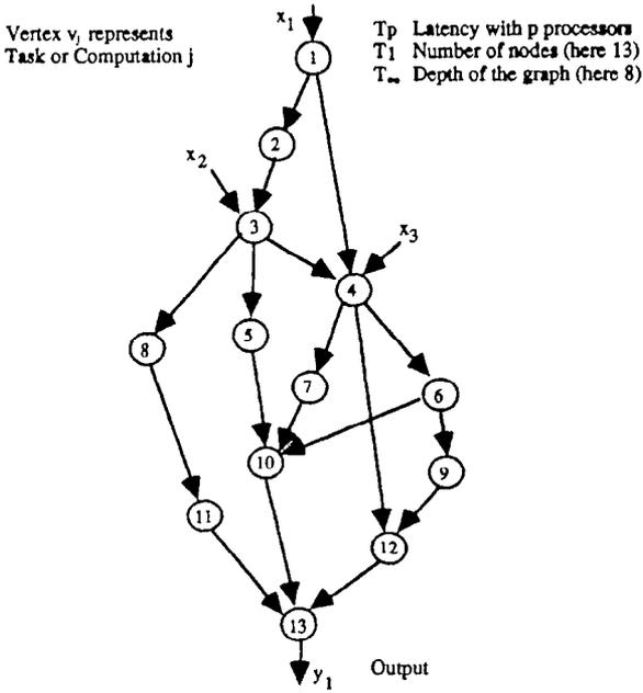
Figure 17.5. Example task system showing communications or dependencies.
