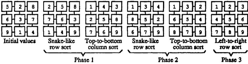
Figure 2.14. The shearsort algorithm on a  $3 \times 3$  mesh.
