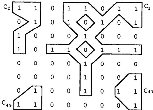
Figure 11.18. Connected components in an  $8 \times 8$  binary image.
