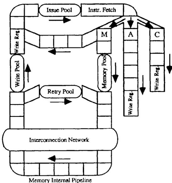
Figure 21.7. The instruction execution pipelines of Tera MTA.
