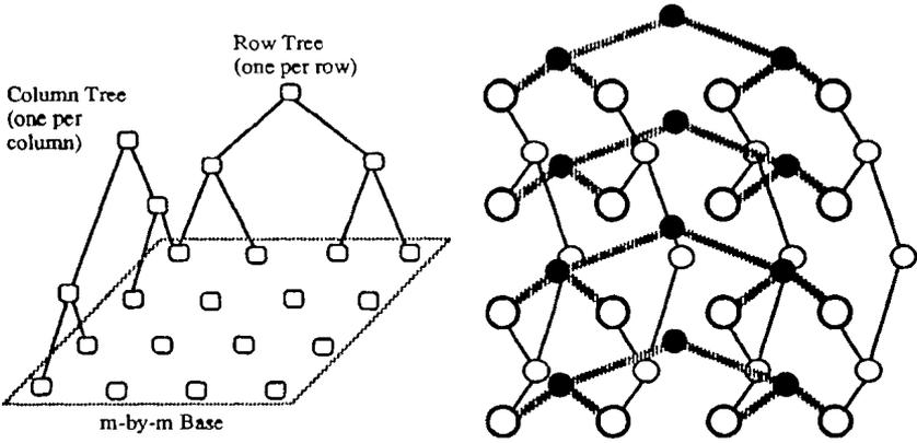
Figure 12.13. Mesh of trees architecture with three levels and a 4x4 base.
