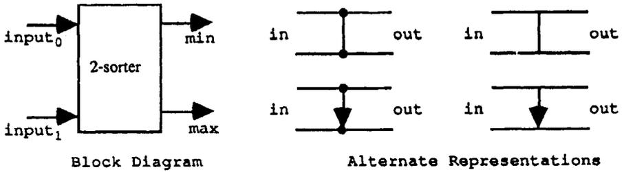
Figure 7.2. Block diagram and four different schematic representations for a 2-sorter.
