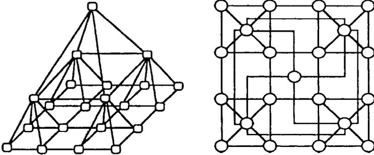
Figure 12.11 Pyramid with three levels and  $4 \times 4$  base along with its 2D layout.
