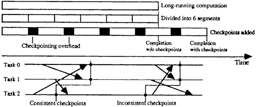
Figure 19.14. Checkpointing, its overhead, and pitfalls.
