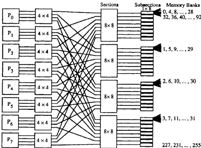
Figure 21.6. The processor-to-memory interconnection network of Cray Y-MP.
