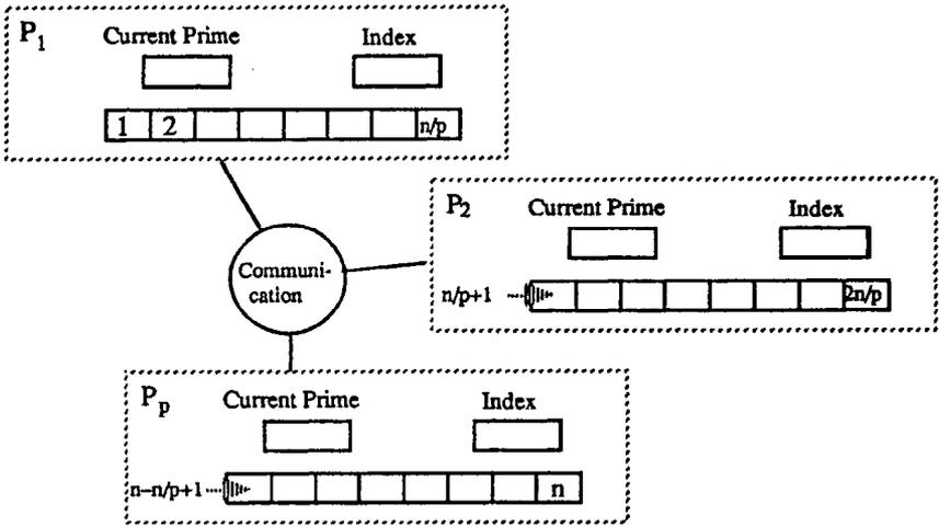
Figure 1.7. Data-parallel realization of the sieve of Eratosthenes.
