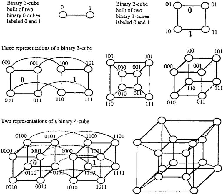
Figure 13.1. The recursive structure of binary hypercubes.
