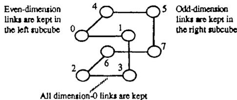
Figure 15.20. Example of a pruned hypercube.
