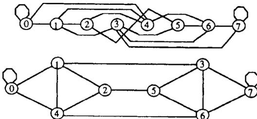
Figure 15.17. Alternate views of an eight-node shuffle-exchange network.
