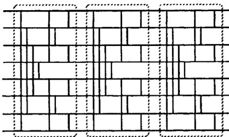
Figure 7.14. Periodic balanced sorting network for eight inputs.
