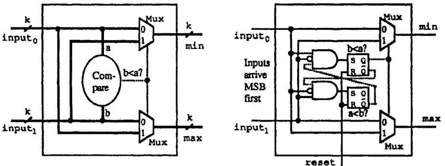
Figure 7.3. Parallel and bit-serial hardware realizations of a 2-sorter.
