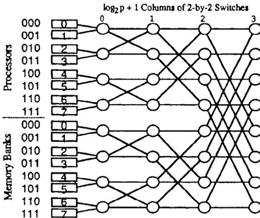
Figure 15.8. Butterfly network used to connect modules that are on the same side.
