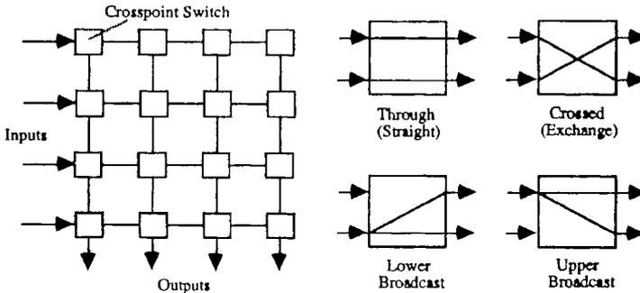
Figure 22.2. Example 4x4 and 2x2 switches used as building blocks for larger networks.
