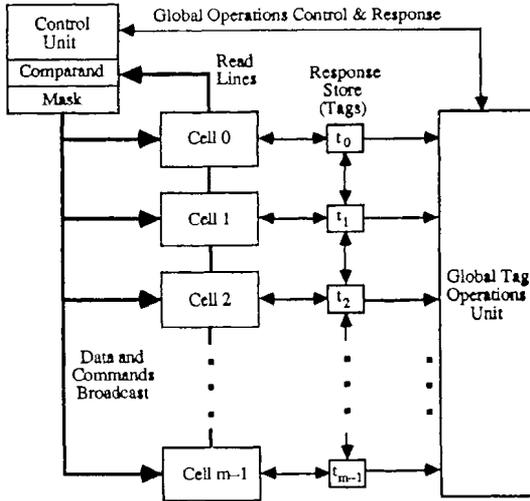
Figure 23.1. Functional view of an associative memory/processor.
