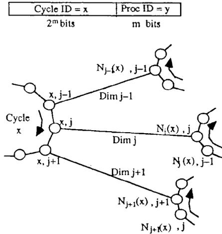
Figure 15.15. CCC emulating a normal hypercube algorithm.
