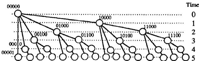
Figure 14.9. The binomial broadcast tree for a 5-cube.
