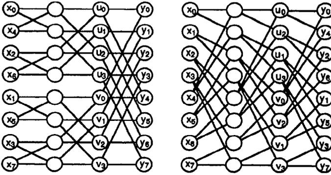
Figure 8.11. Butterfly network for computing an eight-point FFT.
