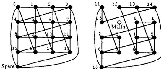
Figure 19.12. Reconfigurable  $4 \times 4$  mesh with one spare.
