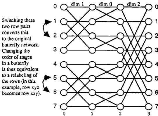
Figure 15.5. Butterfly network with permuted dimensions.
