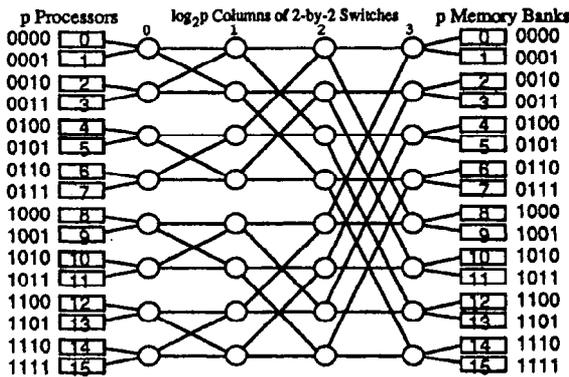
Figure 6.9. Example of a multistage memory access network.
