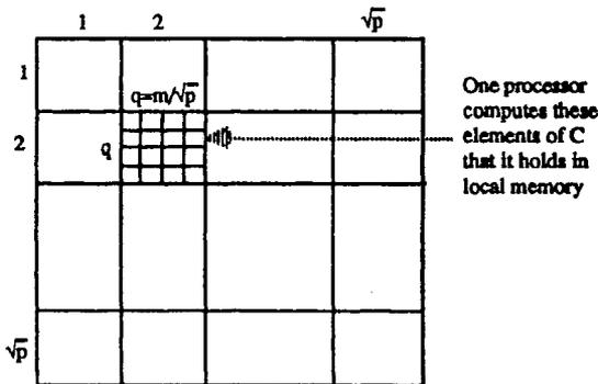
Figure 5.13. Partitioning the matrices for block matrix multiplication.
