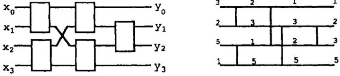
Figure 7.4. Block diagram and schematic representation of a 4-sorter.
