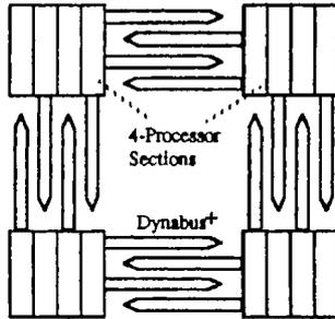
Figure 22.5. Four four-processor sections interconnected by Dynabus<sup>+</sup>.
