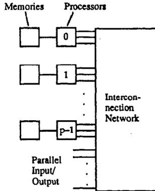
Figure 4.5. A parallel processor with distributed memory.
