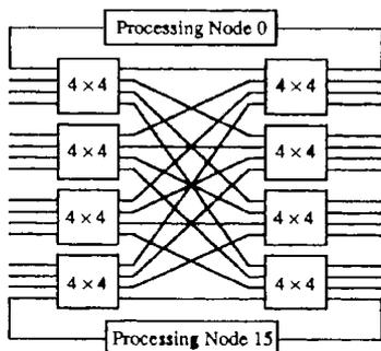
Figure 21.4. A small 16-node version of the multistage interconnection network of the BBN Butterfly.
