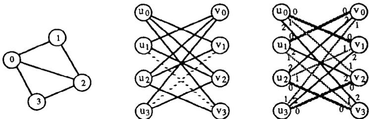
Figure 17.1. Converting a routing step in a degree-3 network to three permutations or perfect matchings.
