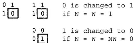
Figure 11.20. Transformation or rewriting rules for Lavialdi's algorithm (no other pixel value changes).
