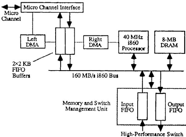
Figure 22.11. The network interface controller of IBM SP2.
