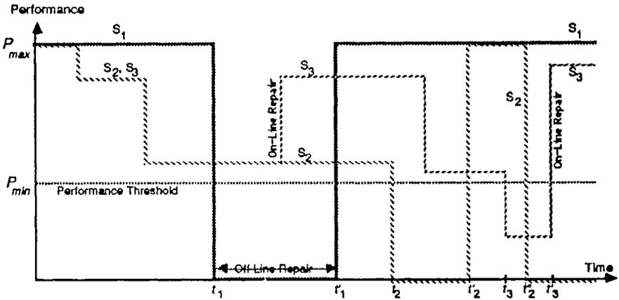
Figure 19.13. Performance variations in three example parallel computers.
