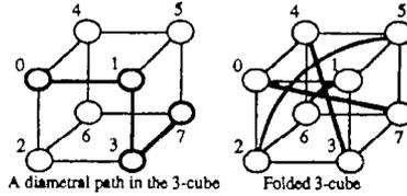
Figure 15.2. Deriving a folded 3-cube by adding four diametral links.
