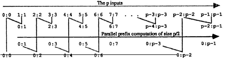
Figure 5.7. Parallel prefix computation using a divide-and-conquer scheme.
