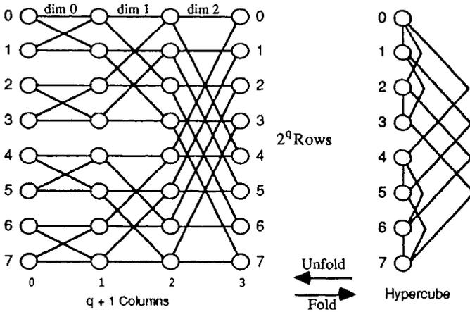
Figure 14.5. Unfolded 3-cube or the 32-node butterfly network.
