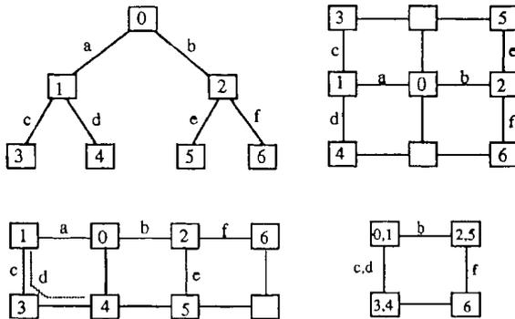
Figure 13.2. Embedding a seven-node binary tree into 2D meshes of various sizes.
