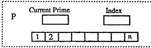
Figure 1.4. Schematic representation of single-processor solution for the sieve of Eratosthenes.
