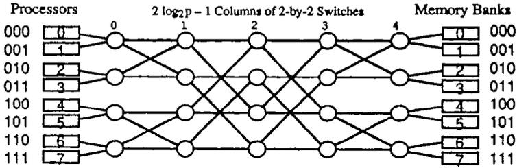
Figure 15.9. Beneš network formed from two back-to-back butterflies.
