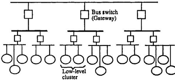
Figure 4.9. Example of a hierarchical interconnection architecture.
