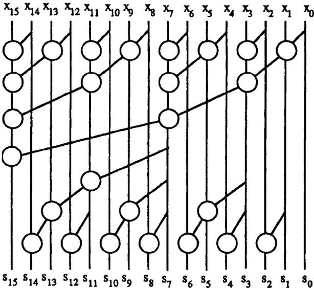
Figure 8.8. Brent–Kung parallel prefix graph for 16 inputs.
