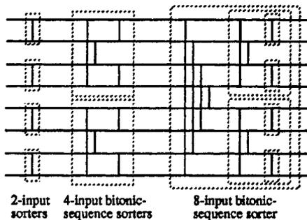
Figure 7.13. Batcher's bitonic sorting network for eight inputs.
