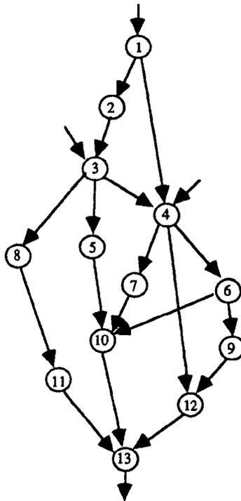
Figure 1.13. Task graph exhibiting limited inherent parallelism.
