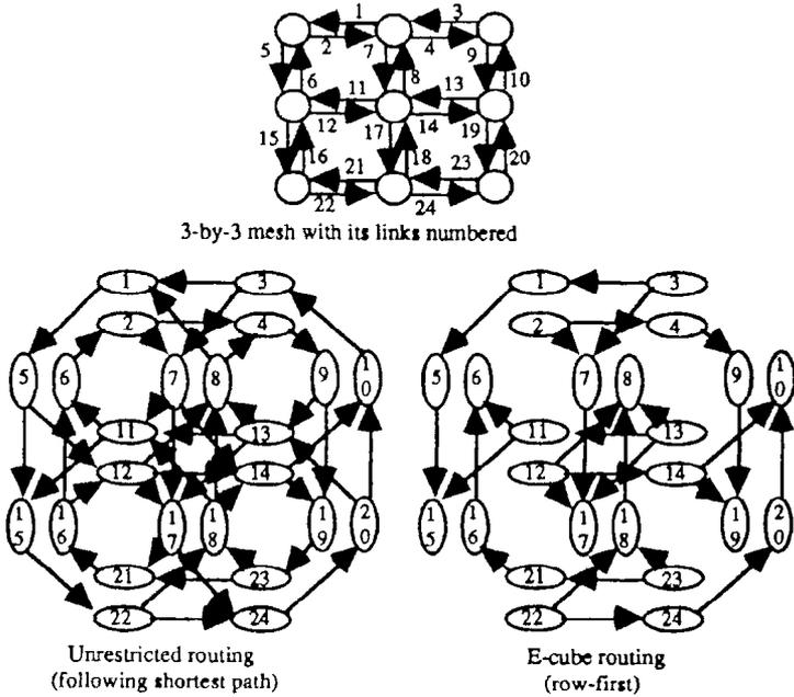
Figure 10.12. Use of dependence graph to check for the possibility of deadlock.
