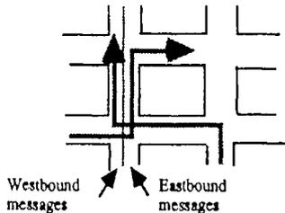
Figure 10.13. Use of virtual channels for avoiding deadlocks.
