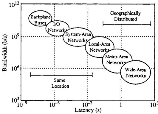
Fig. 24.4. Various types of intermodule and intersystem connections.
