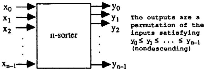
Figure 7.1. An  $n$ -input sorting network or an  $n$ -sorter.
