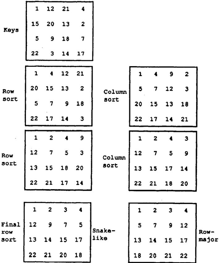
Figure 9.8. Example of shearsort on a 4 x 4 mesh.
