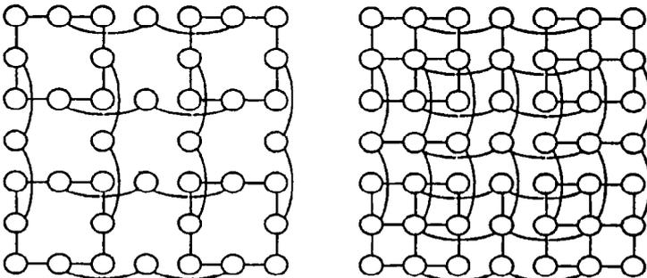
Figure 16.11. Mesh of trees compared with mesh-connected trees.
