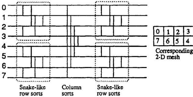
Figure 7.15. Design of an 8-sorter based on shearsort on  $2 \times 4$  mesh.
