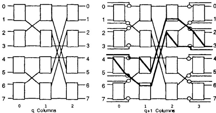
Figure 19.9. Regular butterfly and extra-stage butterfly networks.
