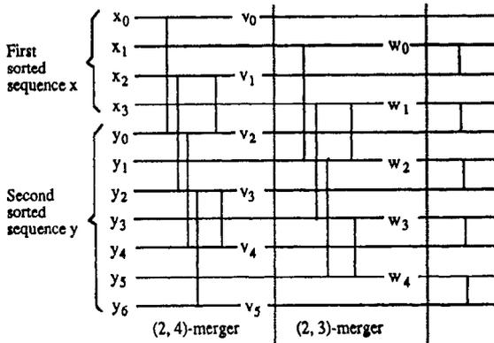
Figure 7.9. Batcher's even-odd merging network for 4 + 7 inputs.
