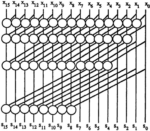
Figure 8.9. Kogge–Stone parallel prefix graph for 16 inputs.
