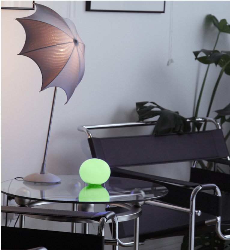
Figure 5.6. The Ambient Orb. The orb can be programmed to change color to reflect the general health of an organization, or to show the status of a specific key indicator.
