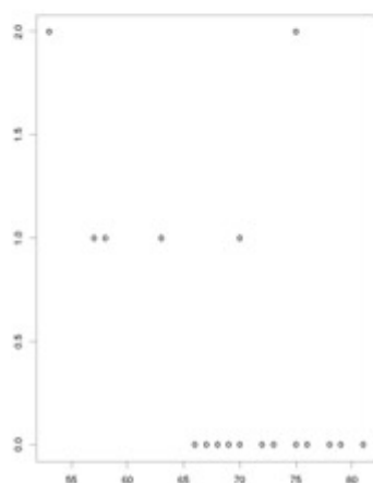
Figure 11.6: Number of O-Rings Damaged (Vertical Axis) against Temperature on Day of Flight, (a) Data Examined before the Flight, and (b) The Complete Data.
