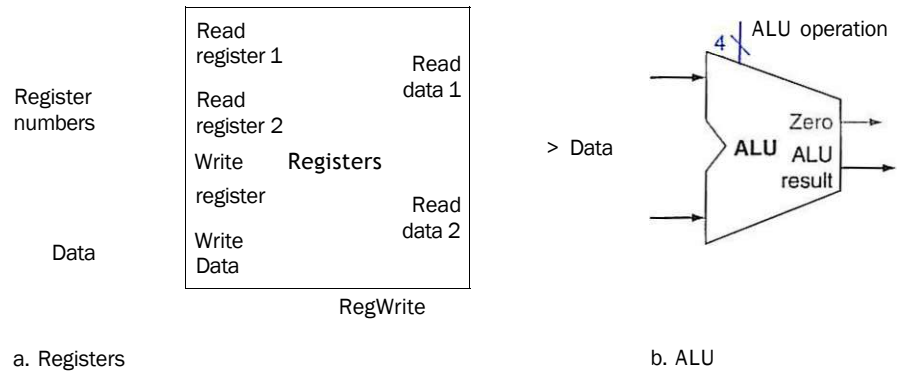
FIGURE 4.7 The two elements needed to implement R-format ALU operations are the register file and the ALU. The register file contains all the registers and has two read ports and one write port. The design of multiported register files is discussed in Section C.8 of Appendix C. The register file always outputs the contents of the registers corresponding to the Read register inputs on the outputs; no other control inputs are needed. In contrast, a register write must be explicitly indicated by asserting the write control signal. Remember that writes are edge-triggered, so that all the write inputs (i.e., the value to be written, the register number, and the write control signal) must be valid at the clock edge. Since writes to the register file are edge-triggered, our design can legally read and write the same register within a clock cycle: the read will get the value written in an earlier clock cycle, while the value written will be available to a read in a subsequent clock cycle. The inputs carrying the register number to the register file are all 5 bits wide, whereas the lines carrying data values are 32 bits wide. The operation to be performed by the ALU is controlled with the ALU operation signal, which will be 4 bits wide, using the ALU designed in Appendix C. We will use the Zero detection output of the ALU shortly to implement branches. The overflow output will not be needed until Section 4.9, when we discuss exceptions; we omit it until then.
