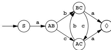
Fig. 5.12. Deterministic automaton for the grammar of Figure 5.6
