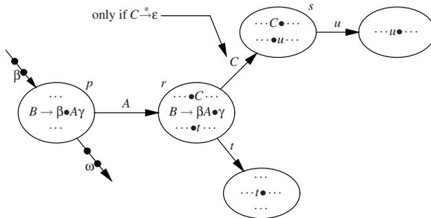
**Fig. 9.38.** Hunting for LALR(1) look-aheads in an LR(0) automaton — the **directly-reads** and **reads** relations
