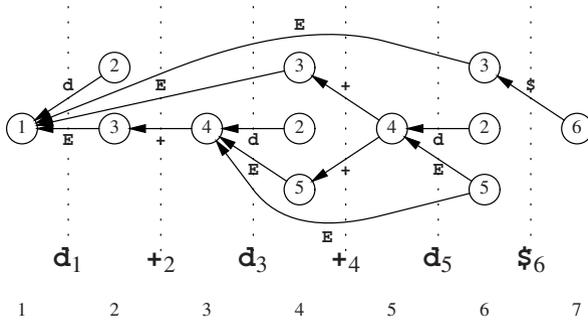
Fig. 11.6. Graph-structured stack for the parsing of  $d+d+d\$$
