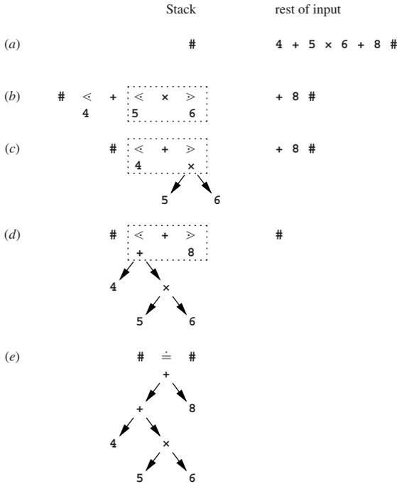
Fig. 9.5. Operator-precedence parsing of  $4+5 \times 6+8$
