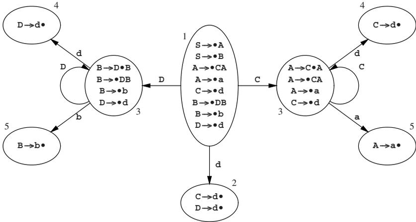
Fig. 9.52. Part of the LR(0) automaton for the grammar of Figure 9.51
