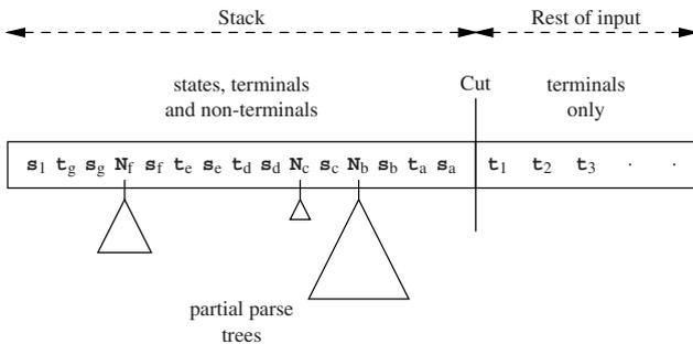
Fig. 9.12. The structure of an LR parse
