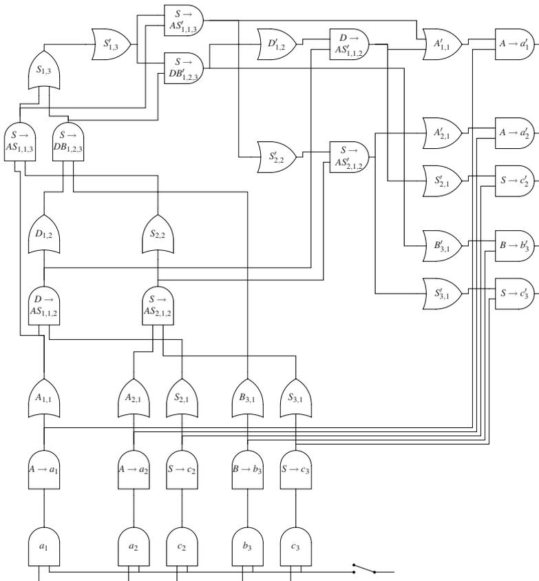
Fig. 14.13. The recognizer/parse-forest circuit for the grammar of Figure 14.9
