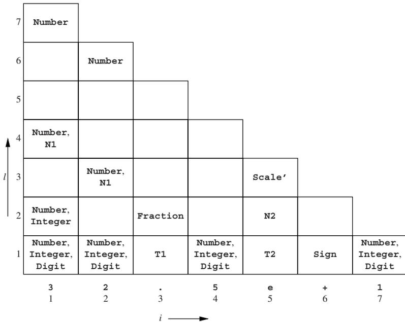
Fig. 4.16. The recognition table for the input sentence 32.5e+1
