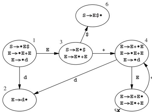
Fig. 11.2. LR(0) automaton to the grammar of Figure 11.1
