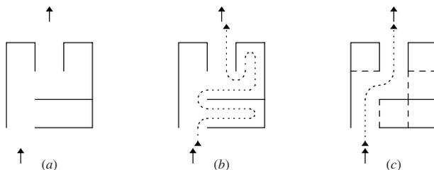
**Fig. 3.10.** A single-exit maze made deterministic by preprocessing
