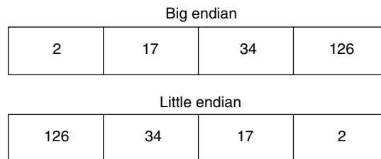
Figure 2.7: Byte ordering sometimes has to be specified when compiling software. The representation of the number 34,677,374 has either of these forms.
