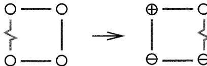
**Figure 9.8:** A small  $\pm J$  spin glass. Via a gauge transformation the aim is to make all bonds ferromagnetic. It fails because the system is *frustrated*.
