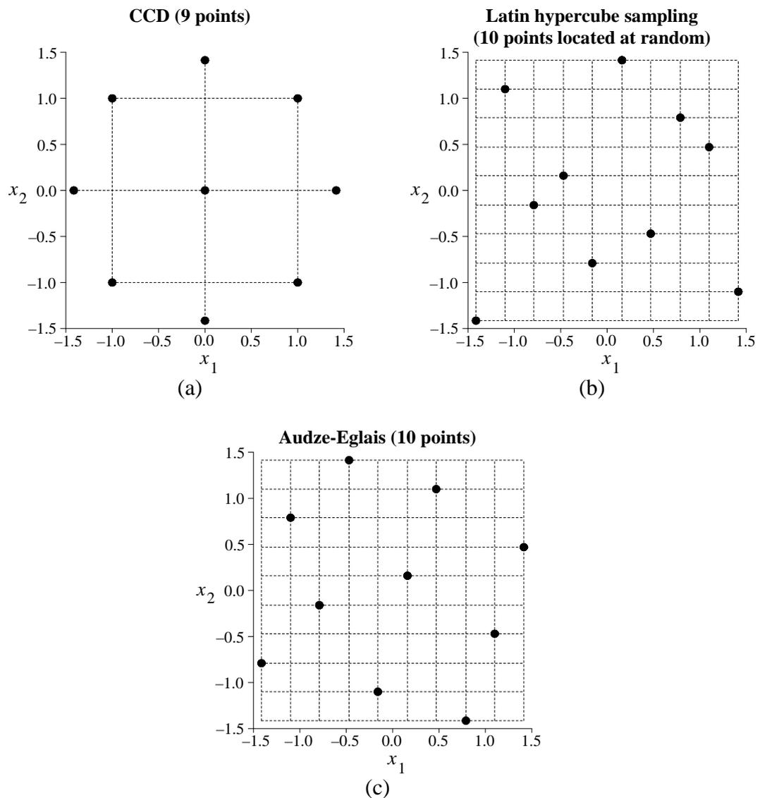
**Figure 3.5** Comparison between CCD (a), Latin hypercube design (b) and Audze-Eglais design (c)
