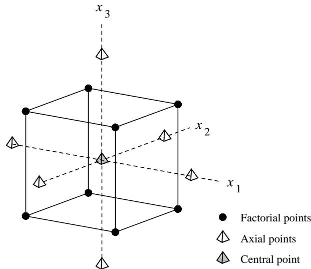
**Figure 3.4** Central composite design for 3 design variables at 2 levels
