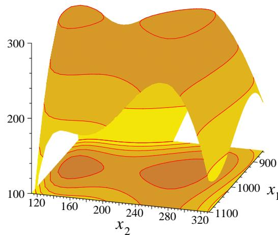
**Figure 3.1** Three-dimensional response surface and the corresponding contour plot for the early age strength of Roman cement where  $x_1$  is the calcination temperature ( $^{\circ}\text{C}$ ) and  $x_2$  is the residence time (mins).
