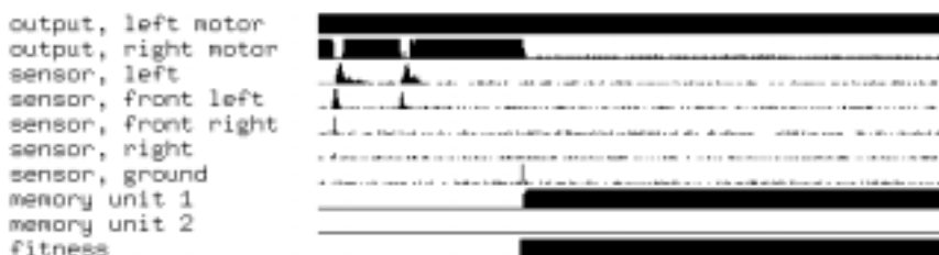
Figure 8. Activation and fitness values during the 400 time steps of the evaluation trial for the robot controller (architecture B) illustrated in Figure 8 (experiment 1). Activation values are illustrated as vertical black lines whose height corresponds to the represented value. All unit activation values lie between 0 and 1 (full height black line) (NB. In the case of the motors 0 corresponds to full speed backward rotation, 0.5 to no motion, and 1 to full speed forward rotation). The fitness value is either 0 (no line), between 0 and 1 (short line), or 100 (full height black line).
