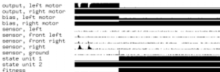
Figure 11. Activation values, motor biases, and fitness points during the 400 time steps of the evaluation trial for the robot controller (architecture D) illustrated in Figure 10 (experiment 1). Biases are shown in the range of -10 (no line) to +10 (full height black line).
