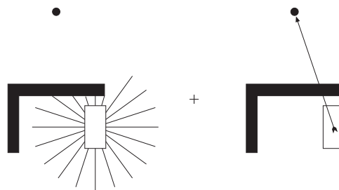
Figure 6. The robot perception: distance from the obstacles (left), relative goal direction (right).
