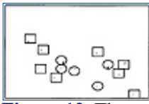
Figure 12 The output image using fuzzy (rule) technique (with attributes A, B, C, and D). Five targets (in circles) and eight false alarms (in squares).
