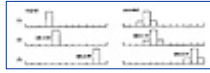
Figure 7 On the left side three different histograms 1, 2, and 3. Since in the SOM, similar vectors are projected to close lying map units, histograms 1 and 2 should be more similar than histograms 1 and 3. However, using Euclidean distance between histograms, this is not so. Instead, the quantization errors (QE) are equal. This is corrected by convoluting the histograms with a symmetric matrix, as seen on the right side.
