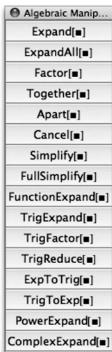
Figure 4.1 The Algebraic Manipulation palette contains many functions that can be used to transform expressions.
