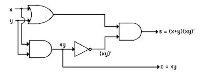
**2.** The gate diagram for a full-adder: A full-adder is a Boolean circuit that adds three bits (x, y), and a carry bit (c) and produces two outputs (a sum bit (c) and a carry bit (c)). The full-adder gate diagram is given in the following figure.
