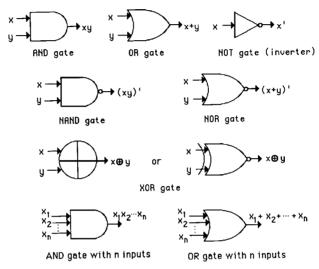
**2.** Gates can be extended to include cases where there are more than two inputs. The figure of Fact 1 also shows an AND gate and an OR gate with multiple inputs. These correspond to  $x_1x_2...x_n$  and  $x_1 + x_2 + \cdots + x_n$ . (Since both operations satisfy the associative laws, no parentheses are needed.)
