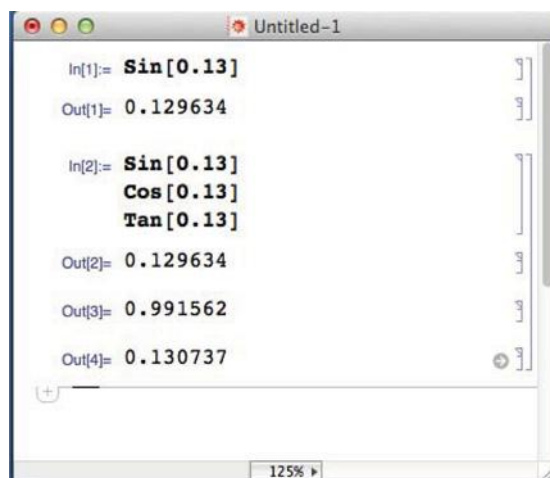
Figure 1.8 Creation of a cell composed of several expressions by using Enter following the first two expressions; that is, for Sin and Cos , and then Shift and Enter after Tan (the Next Computation Suggestions Bar has been hidden)
