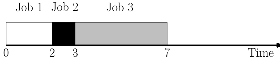
Figure 2.1: An instance of a schedule for the one machine scheduling problem in which p_1 = 2 , r_1 = 0 , p_2 = 1 , r_2 = 2 , p_3 = 4 , r_3 = 1 . In this schedule C_1 = 2 , C_2 = 3 , and C_3 = 7 . If the deadlines for the jobs are such that d_1 = -1 , d_2 = 1 , and d_3 = 10 , then L_1 = 2 - (-1) = 3 , L_2 = 3 - 1 = 2 , and L_3 = 7 - 10 = -3 , so that L_{\max} = L_1 = 3 .
