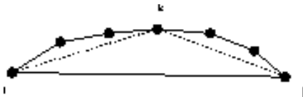
Figure: Selecting the vertex k to pair with an edge (i, j) of the polygon
