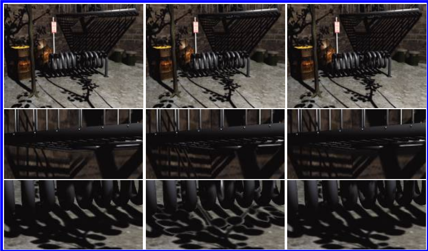
Figure 2.13. Rendering of the same scene using CSM (left), VSM (center), and ESM (right). Main CSM artifacts are near the stairs where shadows fade, and main VSM artifacts are from the light-leaking problems. Image courtesy of Annen et al. [13].
