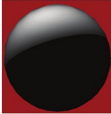
Figure 1.19. Specular cutoff: the specular reflection component spreads where direct light should not reach because the \hat{N} \cdot \hat{L} check was not performed.
