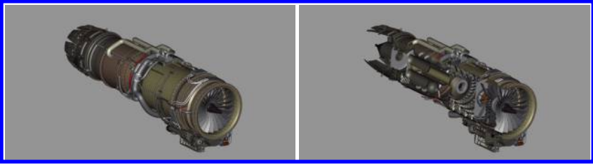
Figure 2.32. A closed model (left) is no longer closed after cross sectioning (right). Image courtesy of NGRAIN (Canada) Corporation.
