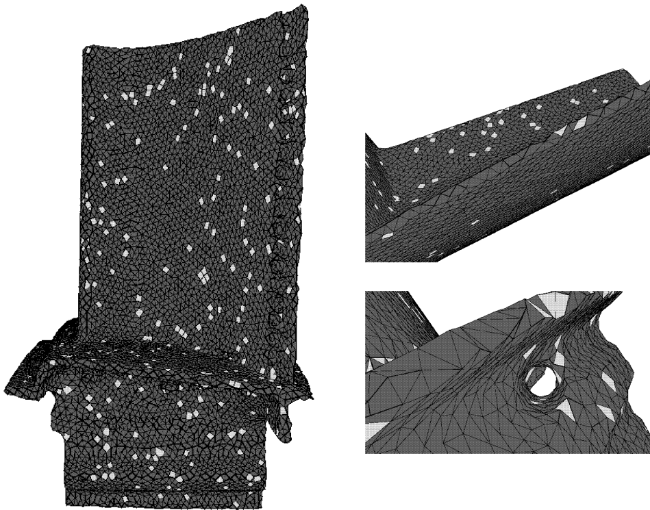
Figure 6: Turbine blade: full view (left), cutting edge and screw hole (right)
