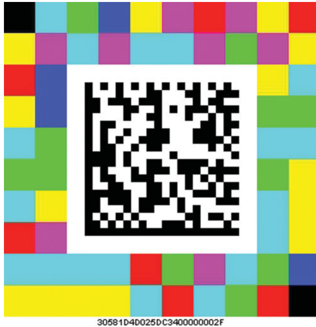
Figure 5.11 Security printing image amenable to componentization through decomposition. The 2D barcode and the white space surrounding it can be extracted and analyzed by a 2D barcode reading pipeline; the surrounding color barcode can be analyzed by a second parallel pipeline; and the microtext below these barcodes can be analyzed by a third parallel pipeline
