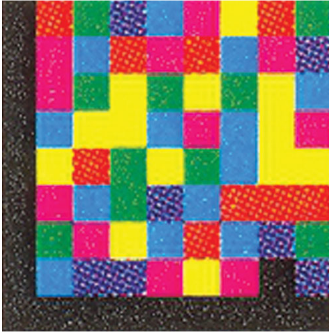
Figure 4.7 Sample 3D (color 2D) barcode that uses a calibrating (nonpayload) indicia approach borrowed from the 2D Data Matrix barcode. All of the perimeter tiles are calibrating. Along the left and bottom sides (with one additional tile near the lower right), the black tiles are used to set the black point and determine orientation and skew. Along the top and right, the six colors used in the payload section—R, G, B, C, M, and Y—are repeated in reading order. The payload consists of 48 color tiles, which in reading order are MCRMRCMMGYGYGYCYCYCMYYRGGYGYMCGBCRRGMYYCRCBCBBMYM
