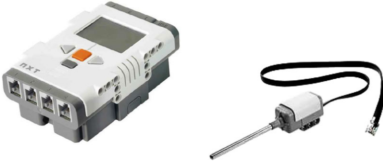
Fig. 7.2 Experimental setup: Lego NXT mindstorms brick (left) and temperature sensor (right)
