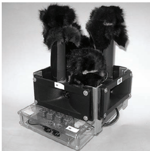
Figure 6. The Acoustic ENSBox's compact microphone array. The four microphones are arranged in a tetrahedral configuration over a 12\text{cm}^2 area.
