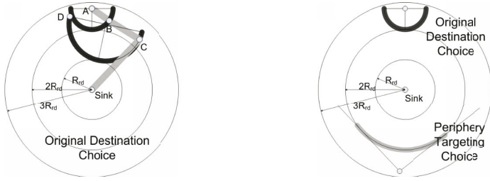
(a) A message from A propagates through B and C to the sink using the original destination choice method
