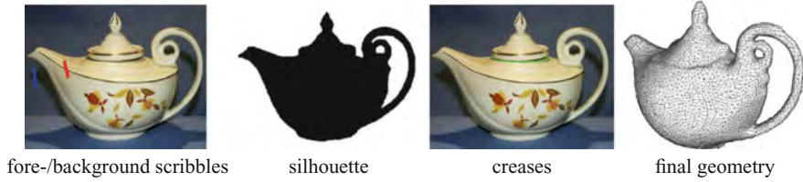
Fig. 16.6 Both methods, Oswald et al. [41] and Töppe et al. [52] have a similar workflow: a silhouette can be estimated with a few user scribbles ( red = foreground, blue = background). Optionally, the user can add creases ( green line ) to locally change the smoothness properties of the final surface. The final geometry shows the discontinuity around the lid and is a result of the method by Töppe et al.
