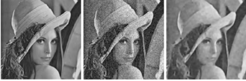
Fig. 9.7 Original, noisy ( \nu = 25 ) and filtered image by MCM ( C = 0.02 , s = 1 , \Delta x = 1 , \Delta t = 0.25 , N = 5 )
