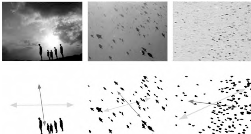
Fig. 7.4 Real images are in the first row. After thresholding, the image components are treated as components of a multi-component shape and then oriented by the method given by Definition 7.2 – the orientations computed are presented by short dark arrows . Long grey arrows represent the orientations computed by the standard method where all components are taken together to build a single shape
