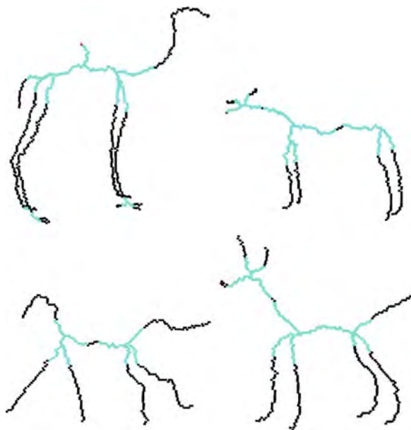
Fig. 6.4 Skeleton partition into simple curves, black , single points, red , and complex sets, light blue
