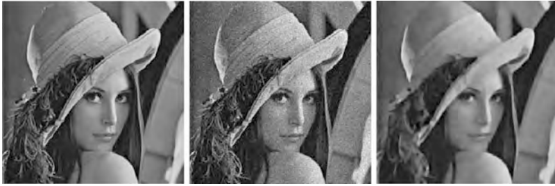
Fig. 9.9 Original, noisy ( \nu = 12 ) and filtered image by AMSS ( C = 0.02, s = 1, \Delta x = 1, \Delta t = 0.2, \rho = (\Delta t)^{1/6}, N = 10 )
