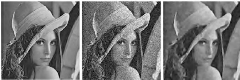
Fig. 9.10 Original, noisy ( \nu = 25 ) and filtered image by AMSS ( C = 0.02, s = 1, \Delta x = 1, \Delta t = 0.25, \rho = (\Delta t)^{1/6}, N = 10 )
