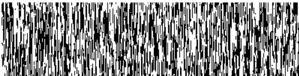
Figure 6.11. A source with low entropy that is not well compressed by Lempel–Ziv. The bit sequence is read from left to right. Each line differs from the line above in f = 5\% of its bits. The image width is 400 pixels.
