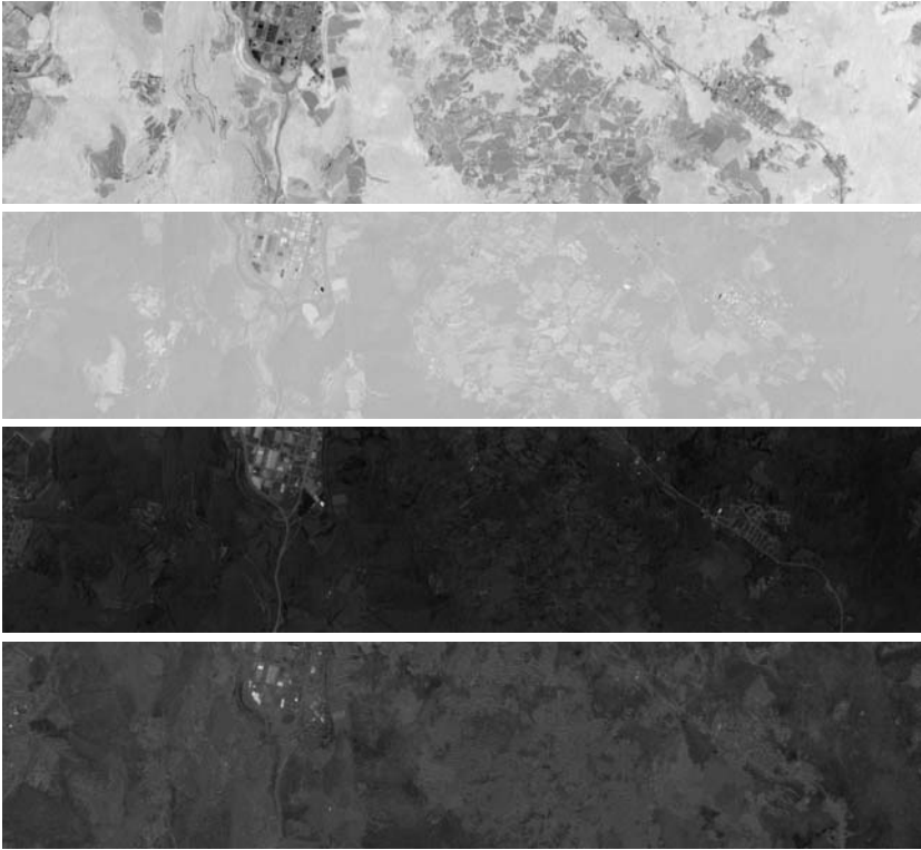
Figure 4.5. Abundance images corresponding to the endmembers discovered by the GA with the morphological independence restriction: GA-MI.
