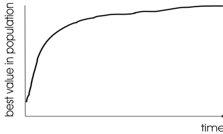
Fig. 2.2. Typical progress of an EA illustrated in terms of development over time of the highest fitness in the population
