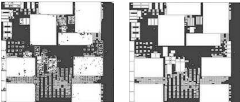
FIGURE 79.2 A global placement (left) with a corresponding detailed placement on a circuit with over one million movable objects. For simplicity, nets are not shown.
