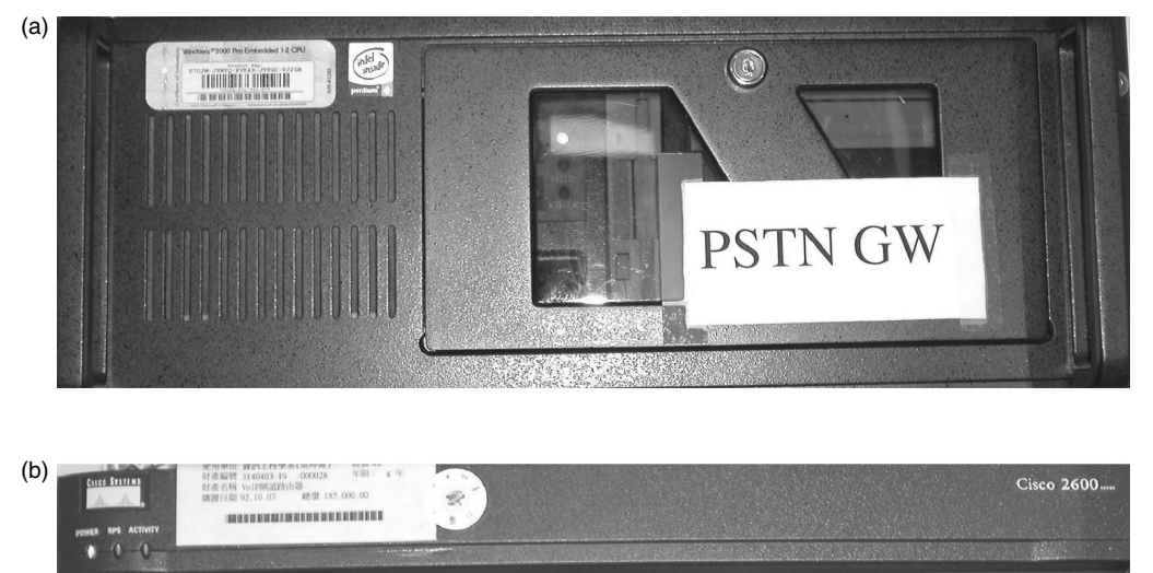
FIGURE 34.3 NTP PSTN gateways: (a) ITRI PSTN gateway; (b) CISCO 2600.
