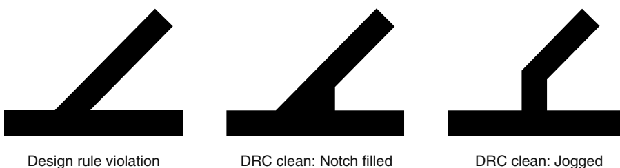
FIGURE 40.12 Illegal and legal angles in the X architecture.
