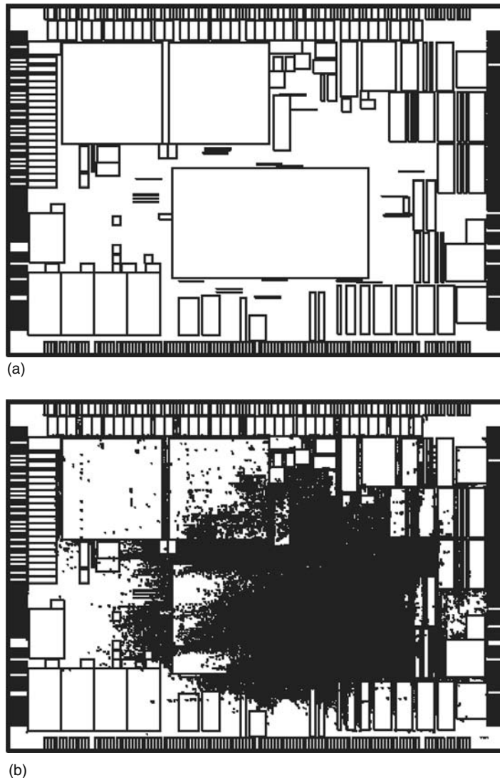
FIGURE 18.12 Illustration of the adaptec2 circuit from the ISPD05 benchmark suite [39] where (a) shows the circuit's fixed obstacles and I/O pads before placement and (b) shows that after the placement of cells after a single QP, many cells may become trapped (or blocked) by fixed obstacles.
