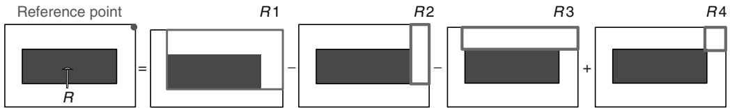
FIGURE 38.6 Convolution lookup for fast lithography simulation. (From Mitra, J., Yu, P., and Pan, D.Z., RADAR: RET-aware detailed routing using fast lithography simulations, in Proceedings of the ACM/IEEE Design Automation , pp. 369–372, June 2005. With permission.)
