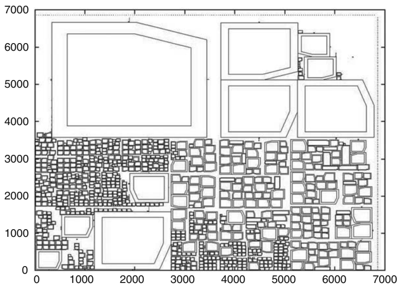
FIGURE 13.3 Block-dominated design, including a few very large blocks that make placement and partitioning very challenging. (Courtesy of Jarrod Roy and the authors of Ref. [26].)
