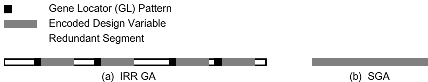
Figure 9.3 Comparison of generic IRR GA and SGA genotype representations. (From Raich & Ghaboussi, in press.)
