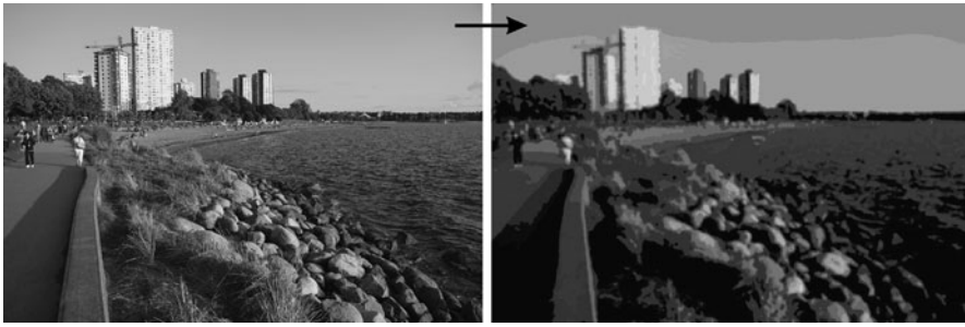
Fig. 9.31 An optimal segmentation according to the Mumford–Shah functional is a description of an image by a non-overlapping set of smooth functions with local support and minimal boundary length. It essentially creates a cartoon-like mapping of the original image with smoothed boundaries
