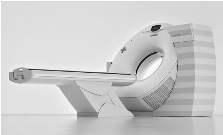
Fig. 2.14 An X-ray CT scanner (Siemens Somatom, image with kind permission by Siemens Sector Healthcare, Erlangen, Germany). Image acquisition takes place in the doughnut-shaped gantry that houses x-ray source and detector rings (which, in this system, can be tilted). The patient is moved through the gantry while slices of CT images are acquired
