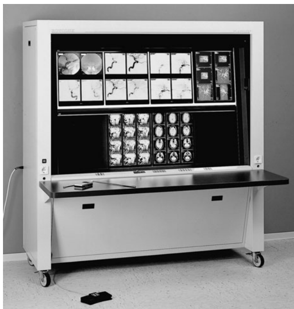
Fig. 3.14 Light box in a traditional reading room: The system can be loaded with several hundreds of films. Films to be read are loaded immediately using a handheld or a foot control (with kind permission of Planilux, Warstein, Germany)
