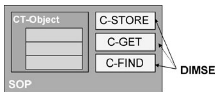
Fig. 3.8 A service-object pair combines an IOD (such as the CT object in this example) with services that are offered for this object. The services are called DICOM Message Service Elements (DIMSE)
