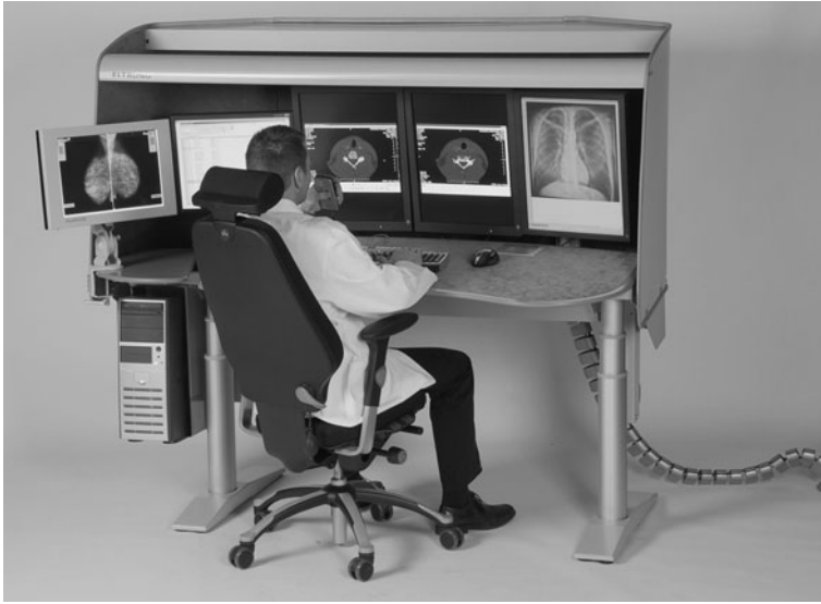
Fig. 3.15 A reading room as part of a PACS displays images on monitors instead of light boxes. Active and passive components of the depicted system control the lighting situation (with kind permission of Planilux, Warstein, Germany)
