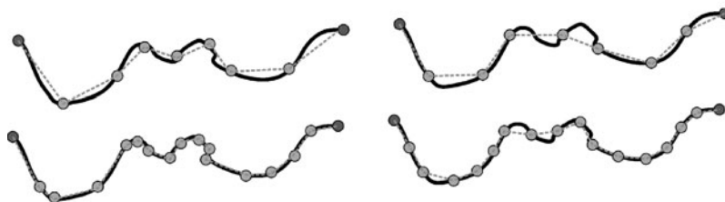
Fig. 11.14 Tertiary landmarks are used to represent curvature of the shape boundary. Sampling may depend on local curvature ( left ) or it may be an even sampling ( right )
