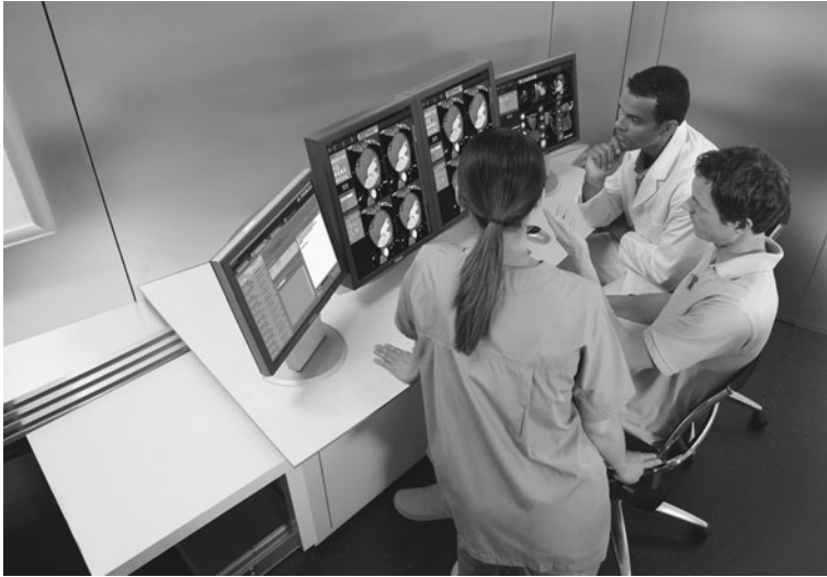
Fig. 3.3 In a PACS, the user has access to images from acquisition systems, workstations and the archive. It usually requires a specific monitor configuration to render images, meta-information, and the interface to administer data access in a suitable way (with kind permission of Siemens Sector Healthcare, Erlangen, Germany)
