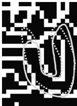
Fig. 11.16 The first step of segmentation with an ASM is to register the shape model with the data accounting for attributes not captured by the ASM such as position, orientation and scale of the model instance
