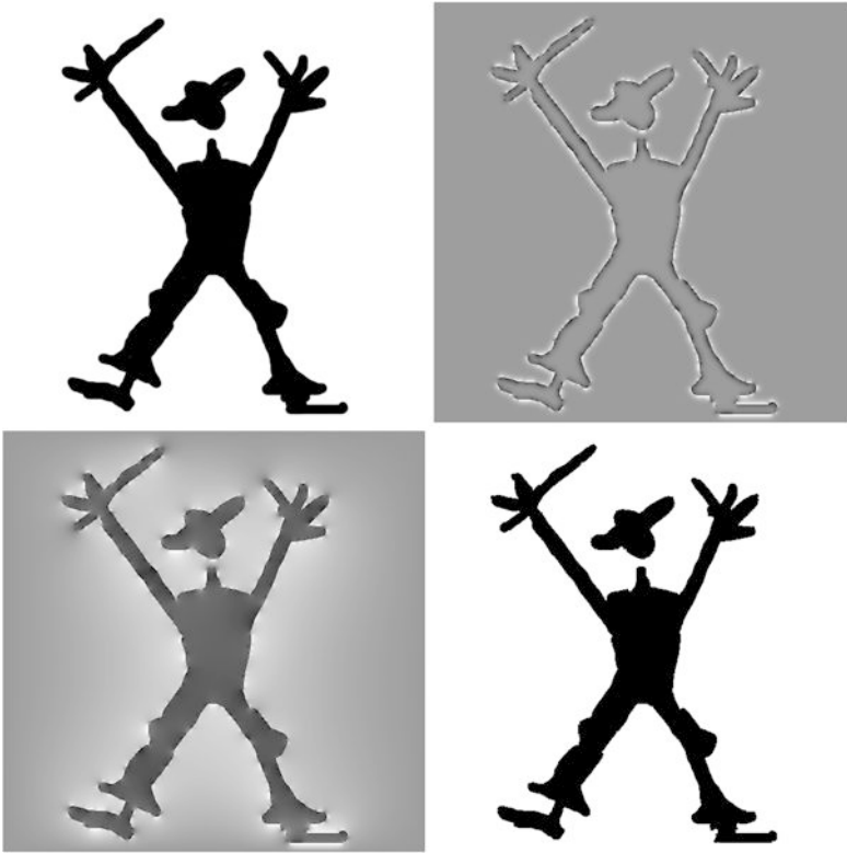
Fig. 17.4 The original image ( top left ) was sampled as described in the text. Solving a discrete version of the Laplace equation with these values as constraints, we obtain the top right image after 100 iterations, the bottom left image after 50000 iterations. Thresholding the bottom left image produces a fairly good reconstruction shown bottom right
