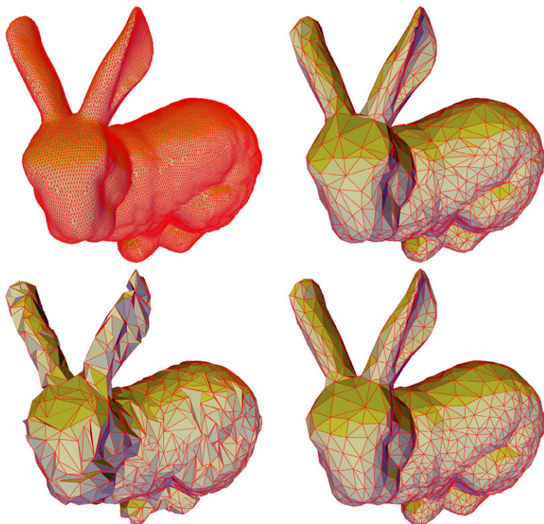
Fig. 11.4 Four bunnies. The top left image shows the Stanford Bunny. To the right it has been simplified using the Garland–Heckbert method with 33000 edge collapses. On the bottom left , 33000 random collapses were used, and on the bottom right 33000 edge collapses with optimal point placement
