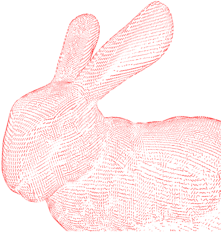
Fig. 8.8 The min curvature directions of the bunny. The directions were estimated using the dihedral angle method from Sect. 8.4. The shape operators at each vertex were averaged with their neighbors to smoothen the field, and then the eigensolutions were found as discussed in Sect. 8.6
