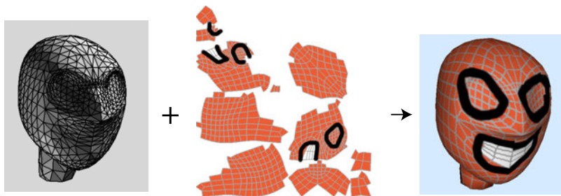
Fig. 10.1 This figure illustrates the principle of texture mapping. Texture stored in a planar image is mapped onto the mesh
