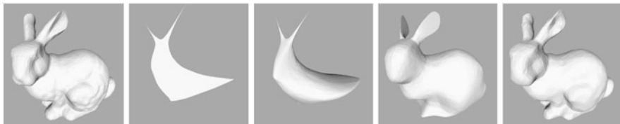
Fig. 9.5 The vertex positions of the original ( simplified ) bunny mesh ( far left ) were projected onto the eigenvectors of the Laplace–Beltrami operator. From this representation, we reconstructed the mesh using 2, 4, 50, and 500 eigenvectors as shown from left to right
