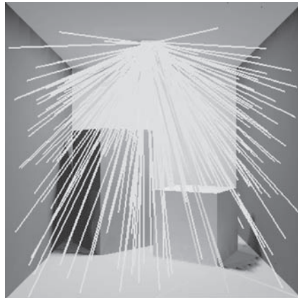
Figure 16.18. The fraction of local lines hitting a particular destination patch is an estimate for the form factor between source and destination.
