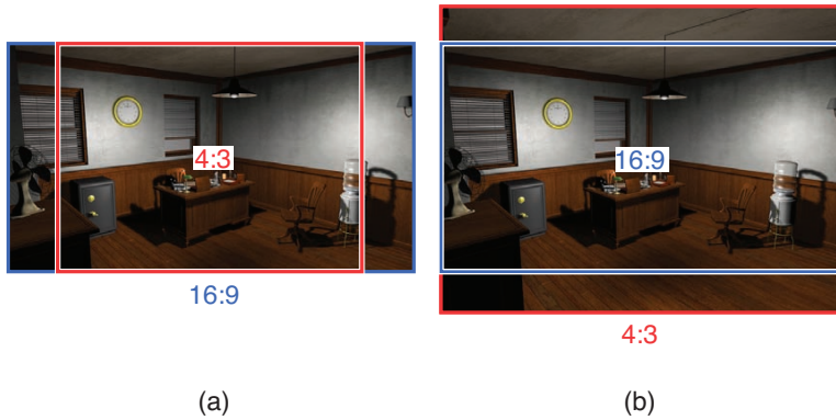
Figure 8.6 16:9 has a wider horizontal FOV (a) and a narrower vertical FOV (b).
