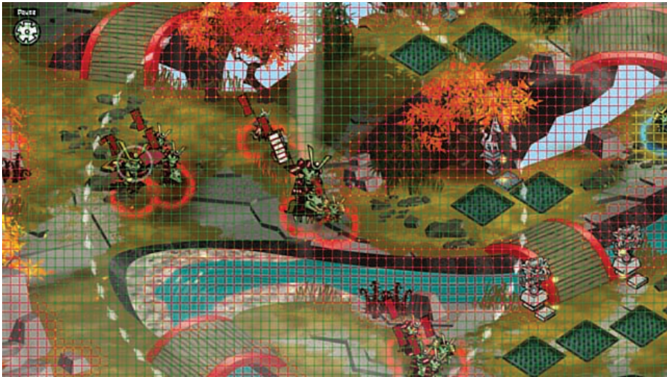
Figure 9.3 Skulls of the Shogun with its AI debug mode enabled to illustrate the square grid it uses for pathfinding.
