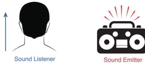
Figure 6.2 Sound listener and emitter; in this case, the sound effect should be heard on the right.
