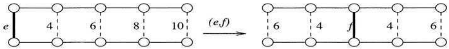
Fig. 3. All edge weights are equal to 1 and the numbers indicated on the chords correspond to the costs of the corresponding fundamental cycles. The cut on the left has a difference between the cheapest and the most expensive cycles of 10 - 4 = 6 ; after the edge swap the difference amounts to 6 - 4 = 2 .
