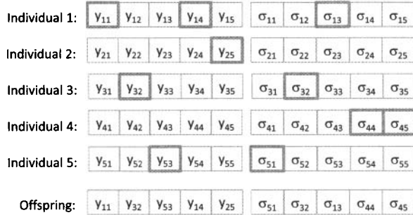
Figure 6.7 Intermediate sexual crossover in an ES, where the problem dimension n = 3 . Each solution feature and standard deviation in the child is half way between the two parents.
