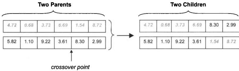
Figure 3.9 Illustration of crossover in a continuous-domain GA. The crossover point is randomly chosen. The two parents produce two children.
