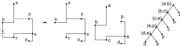
Rectilinear Steiner Tree, Figure 1 Edge substitution by Borah et al.
