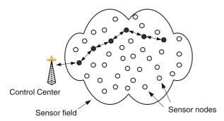
Probabilistic Data Forwarding in Wireless Sensor Networks, Figure 1
