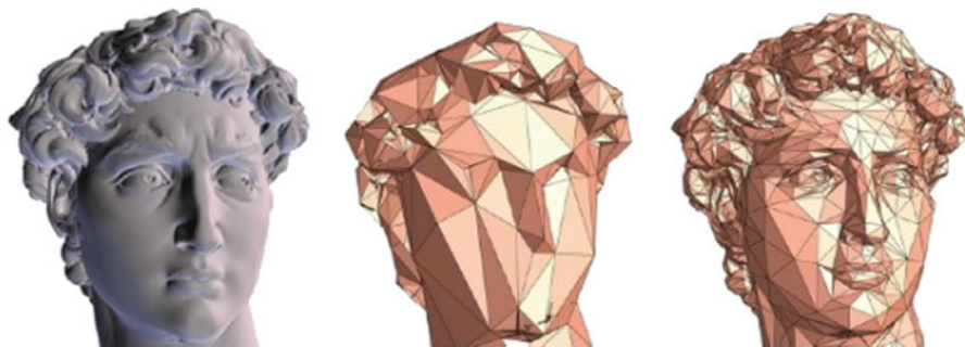
Fig. 8.2 Triangulation generates holes by Z. Wood: a A picture without holes using 1 million triangles, b A picture with 15,000 triangles and 957 holes, and c A picture with 15,000 triangles after deleting all holes
