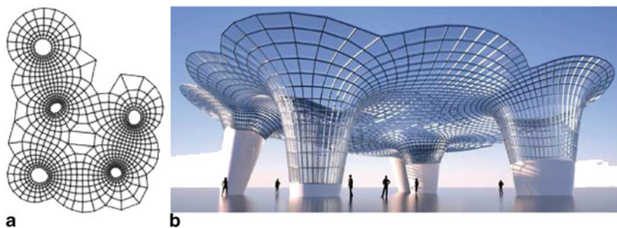
Fig. 13.5 Conforming mapping for geometric design by Y. Yang et al.: a planar design, and b the 3D realization
