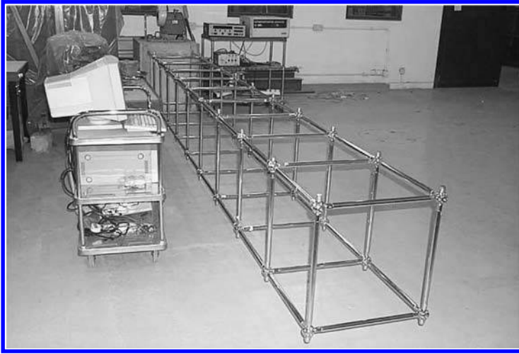
Figure 3.13 Ten-bay cantilever frame structure
