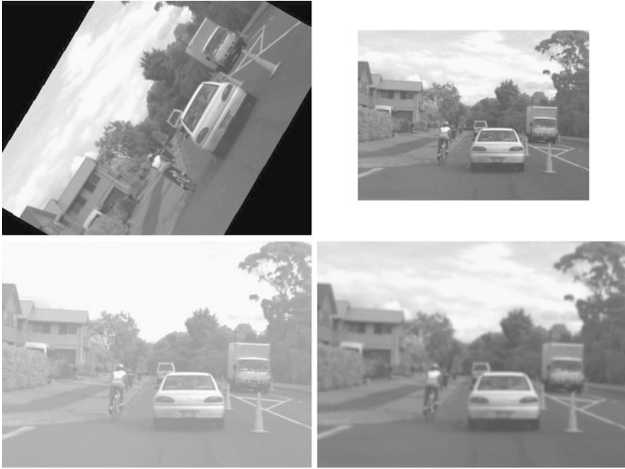
Fig. 9.13 Top, left: A rotated image; the original frame from the sequence bicyclist from EISATS is 640 \times 480 and recorded at 10 bit per pixel. Top, right: A demagnified image. Bottom, left: Uniform brightness change. Bottom, right: A blurred image
