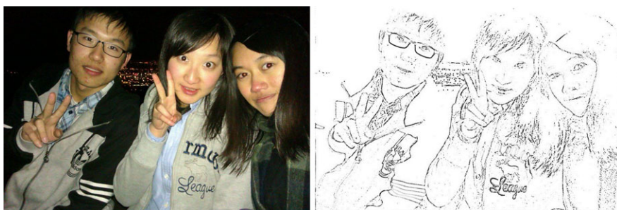
Fig. 1.24 Left: Original image AnnieYukiTim. Right: Edge map resulting when applying the Kovesi algorithm
