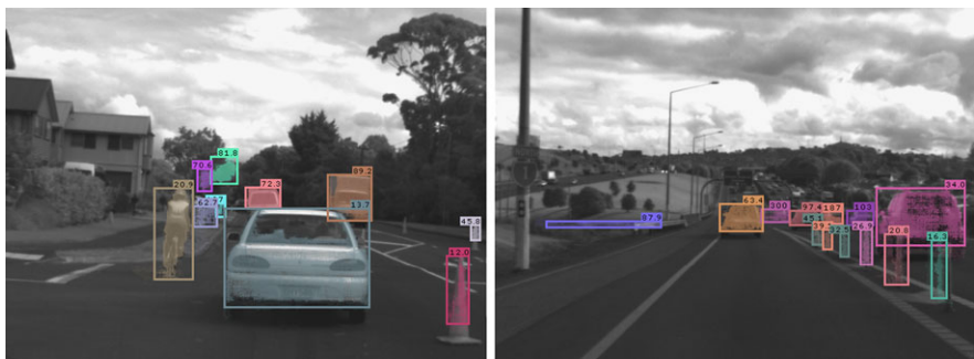
Fig. 5.33 Bounding boxes of tracked segments for video sequences bicyclist and motorway
