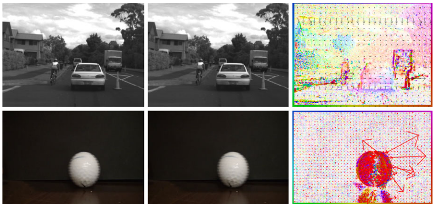
Fig. 4.5 Top, left, and middle: Two subsequent frames of video sequence bicyclist , taken at 25 fps. Top, right: The colour-coded motion field calculated with the basic Horn–Schunck algorithm. Additionally to the colour key, there are also some sparse (magnified) vectors illustrated as redundant information, but for better visual interpretation of the flow field. Bottom, left, and middle: Two subsequent frames of video sequence tennisball . Bottom, right: The colour-coded motion field calculated with the basic Horn–Schunck algorithm
