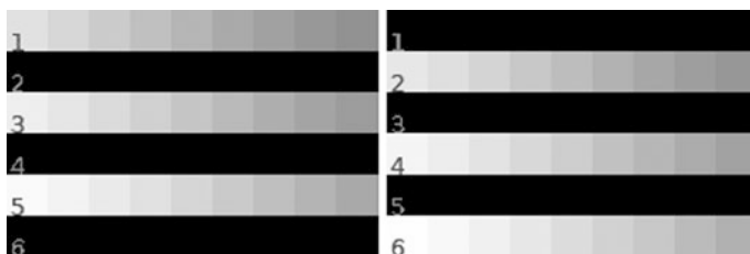
Fig. 6.4 Half-frames defined by either odd ( left ) or even ( right ) row indices
