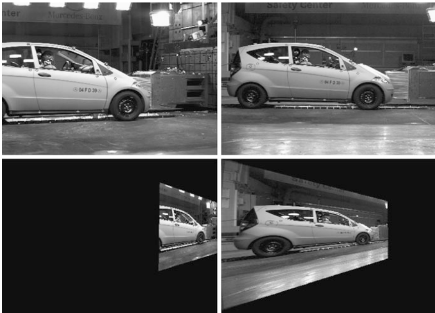
Fig. 6.19 Top: Images recorded by two cameras with significant differences in extrinsic parameters and also (insignificant) differences in intrinsic parameters. Bottom: Two geometrically rectified images taken at different viewing locations by two cameras installed in a crash-test hall
