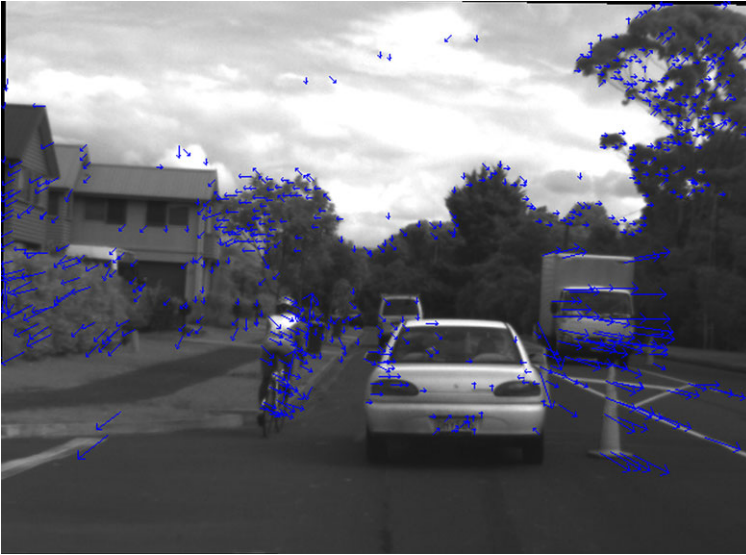
Fig. 4.15 We refer to the same two subsequent frames of a recorded image sequence as shown in Fig. 4.5. The optical flow calculated with original Lucas–Kanade algorithm; k = 25 for a 5 \times 5 neighbourhood
