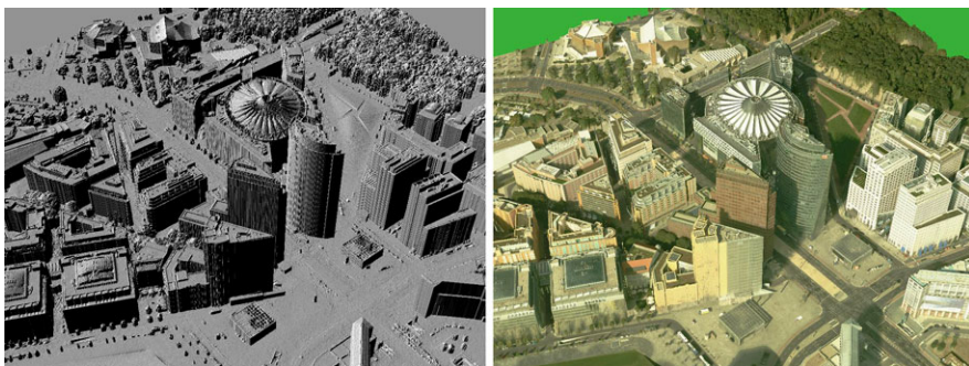
Fig. 7.1 Left: Surfaces reconstructed from image data recorded in an airplane. Right: Surfaces after texture mapping using recorded images. The scene shows the Sony Centre at Berlin, Germany
