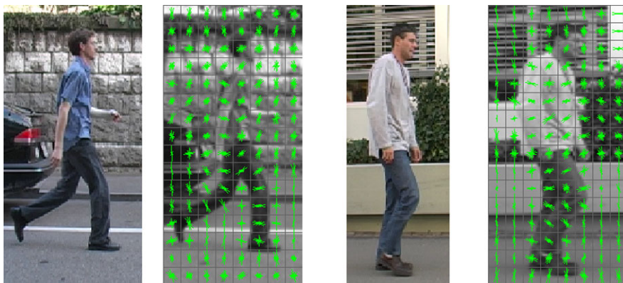
Fig. 10.8 The length of vectors in nine different directions in each cell represents the accumulated magnitude of gradient vectors into one of those nine directions
