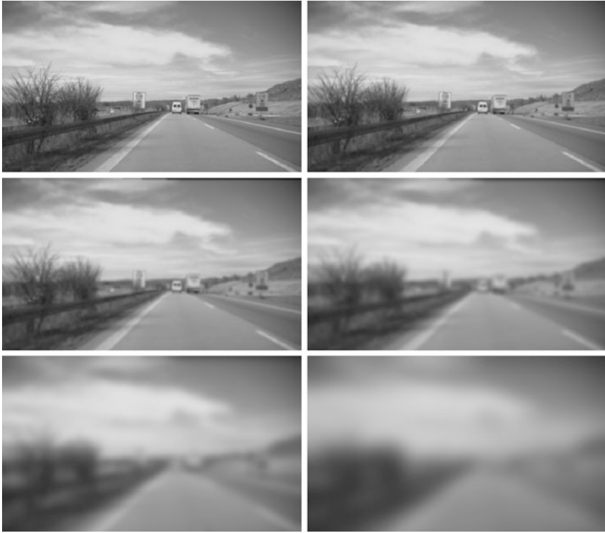
Fig. 2.14 Smoothed versions of the image Set1Seq1 (shown in Fig. 2.4, upper left) for \sigma = 0.5 , \sigma = 1 , \sigma = 2 , \sigma = 4 , \sigma = 8 , and \sigma = 16 , defining six layers of the Gaussian scale space
