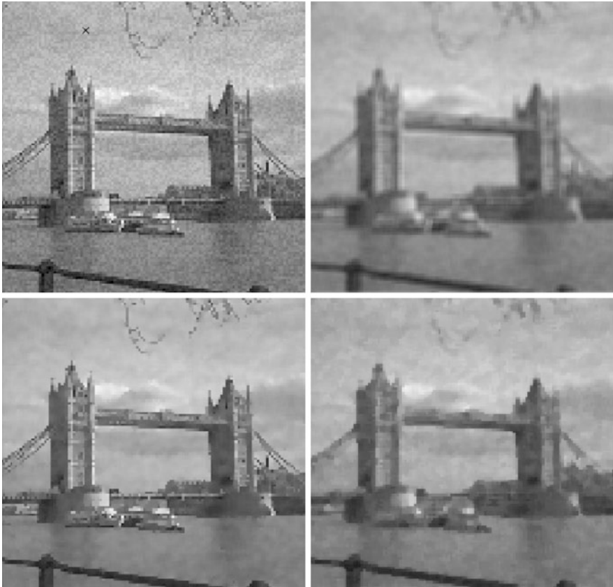
Fig. 2.15 Illustration of noise removal. Upper left: 128 \times 128 input image with added uniform noise ( \pm 15 ). Upper right: 3 \times 3 box filter. Lower left: 3 \times 3 sigma-filter with \sigma = 30 . Lower right: 3 \times 3 median filter
