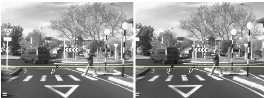
Fig. 8.1 A stereo pair Crossing . Starting at pixel location p in the left image, we search along the epipolar line for a corresponding pixel location q . How to detect q (e.g. in a homogeneously textured region as shown here)? A correct q would be to the right of the shown q
