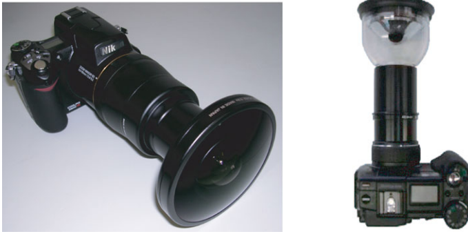
Fig. 6.12 Omnidirectional cameras. Left: A fish-eye camera. Right: A digital camera with a hyperboloidal-shaped mirror
