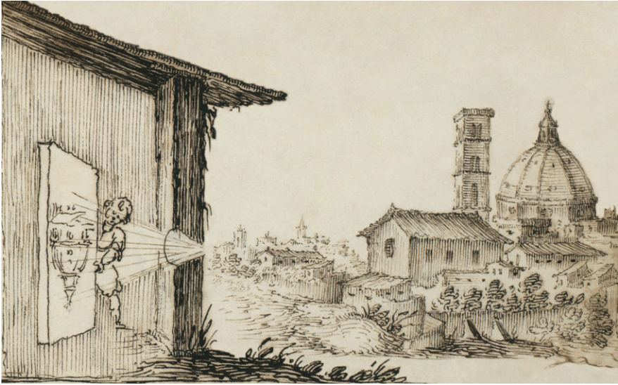
Fig. 6.1 A drawing (in the public domain) of a camera obscura in the 17th century “Sketchbook on military art, including geometry, fortifications, artillery, mechanics, and pyrotechnics”. Outside objects are projected top-down through a small hole onto a wall in the dark room
