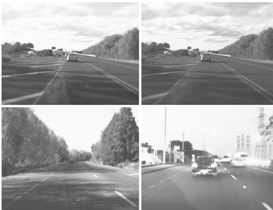
Fig. 2.24 Example images from real-world scenes ( black pixels at borders are caused by image rectification, to be discussed later in the book). The pair of images NorthLeft and NorthRight in the top row show illumination differences between time-synchronized cameras when the exposures are bad. The bottom-left image LightAndTrees shows an example where trees can cause bad shadow effects. The bottom-right image MainRoad shows a night scene where head-lights cause large bright spots on the image
