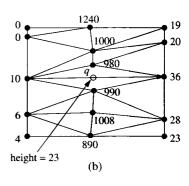
Figure 9.3 Flipping one edge can make a big difference
