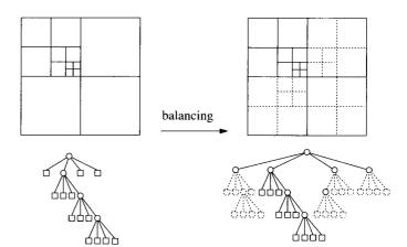
Figure 14.5 A quadtree and its balanced version
