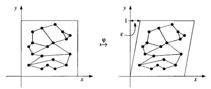
Figure 6.9 The shear transformation
