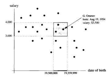
Figure 5.1 Interpreting a database query geometrically
