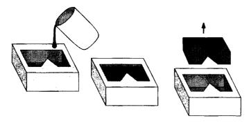
Figure 4.1 The casting process
