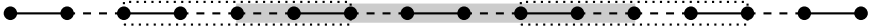
Fig. 6.1. An augmenting path (indicated by gray area) and environments of possible mutations leading to extensions or shortenings (dotted)
