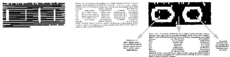
Fig. 5.7 Application of RLSA (on the left) and of RLSO (on the right) to the non-Manhattan digitized document in the middle. Below, the three text frames identified by RLSO
