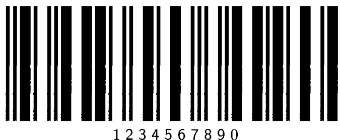
Figure 5.4 Interleaved two out of five
