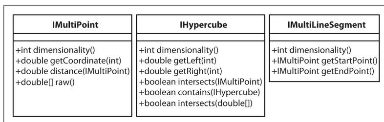
Figure 9-2. Interfaces to represent multiple dimensional data
