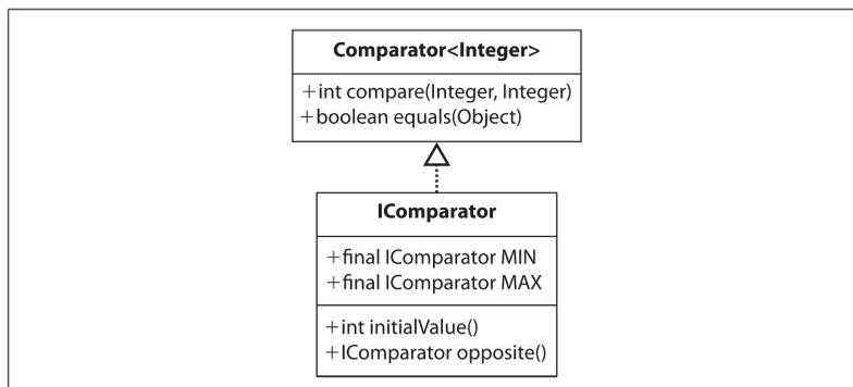
Figure 7-16. *IComparator* interface abstracts *MAX* and *MIN* operators
