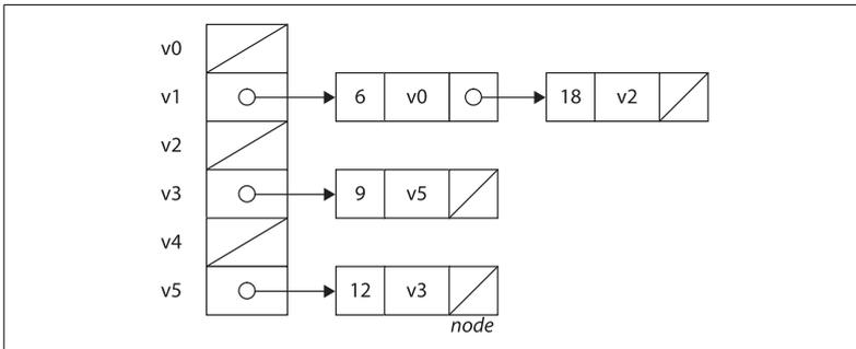
Figure 6-3. Adjacency list representation of directed, weighted graph
