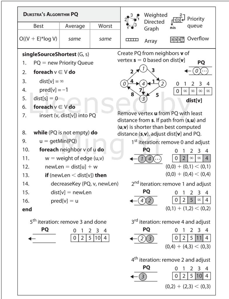
Figure 6-13. Dijkstra's Algorithm with priority queue fact sheet
