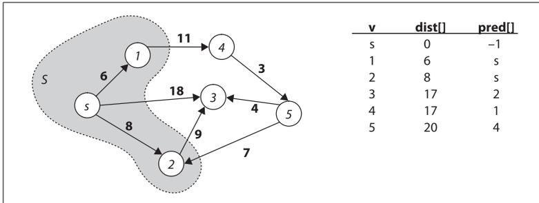
Figure 6-14. Dijkstra's Algorithm expands the set  $S$
