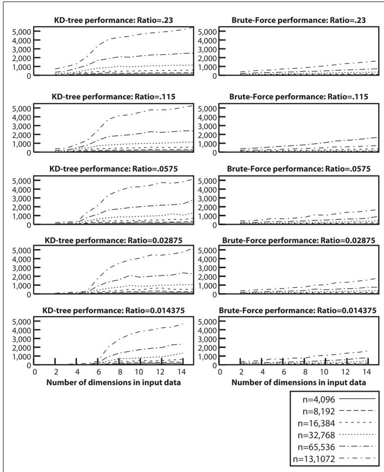
Figure 9-26. Comparing kd-tree versus brute force for situation 2
