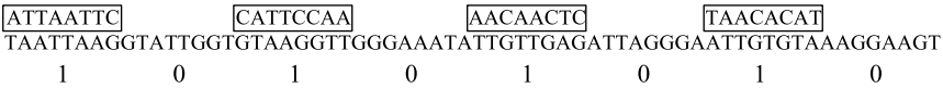
Figure 9.3 Illustration of the stickers model that encodes 10101010. Note that the memory strand consists of eight eight-basis-long subsections. Each subsection is defined as 1 by annealing a sticker and defined as 0 by annealing no sticker.
